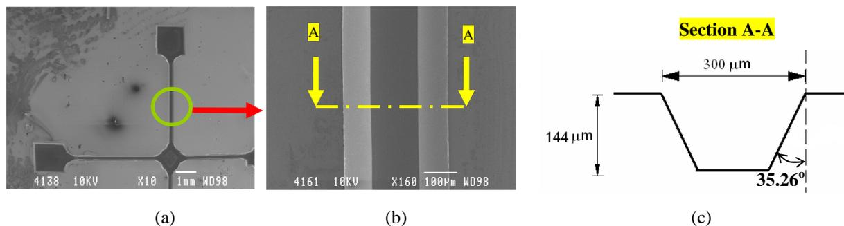
**Figure 5:** (a) Smooth sidewalls of the inlet port produced by the anisotropic etching (b) Mixing zone of the microfluidic channel.
