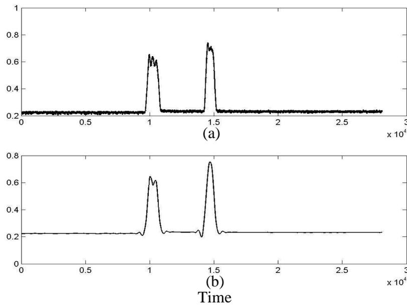
**Figure 10.** Response of the sensor to a passing vehicle: (a) the original signal; (b) the de-noised signal.
