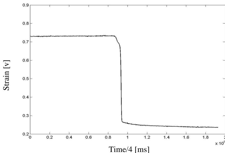
**Figure 8.** Response of the sensor after an applied force vanishes.
