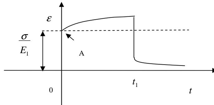
**Figure 6.** Strain curve for Maxwell-Kelvin model.
