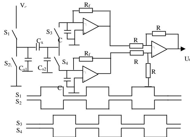
**Figure 3.** Measuring circuit and switching wave forms, with stray capacitances shown ( $C_{s1}$ ,  $C_{s2}$ ).
