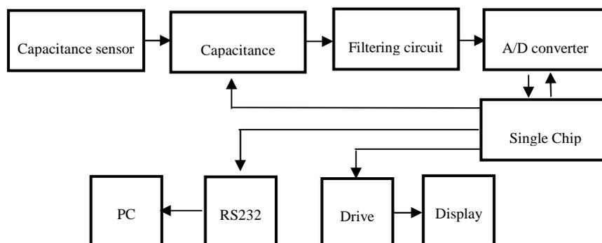
**Figure 2.** Block diagram of measuring circuit.
