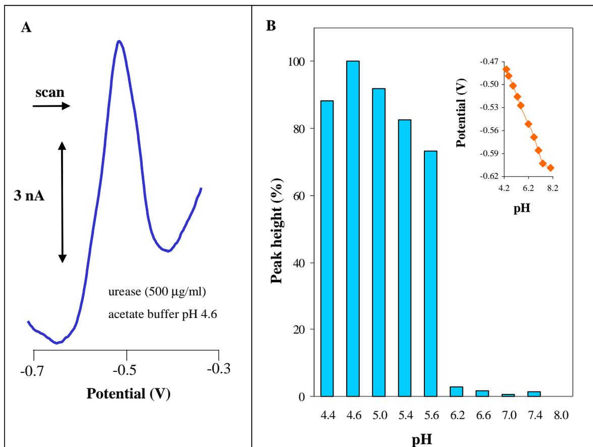
**Figure 4.** Differential pulse voltammogram of urease ( $500 \mu\text{g/ml}$ ) measured in the presence of acetate buffer ( $0.2$  M, pH  $4.6$ ) and accumulation time of  $120$  s (A). Changes in urease peak height in the presence of acetate (pH of  $4.4 - 5.6$ ) and phosphate buffer (pH of  $6.2 - 8.0$ ); in inset: the influence of pH on potential of the peak (B).
