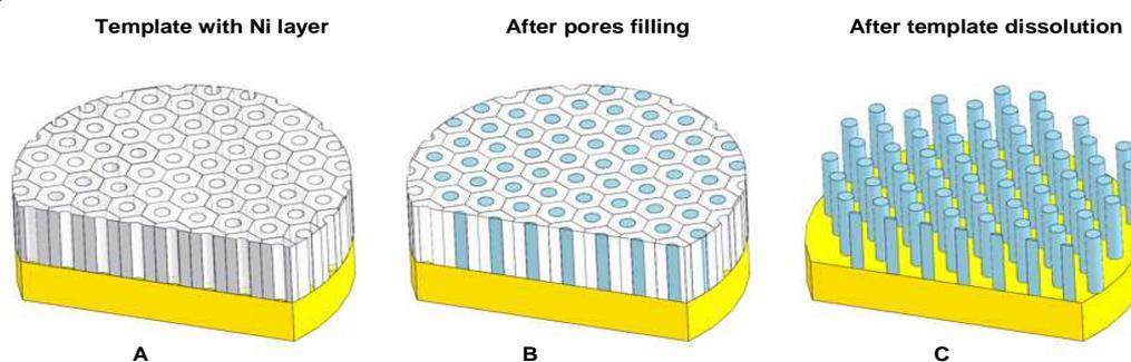
**Figure 1.** Whatman Anodisc as the template with sputtered Ni layer on the bottom (A), nanopores filled with Ni nanocrystal undergalvanostatic conditions (B), Ni nanopillars obtained after dissolution of the template (C).
