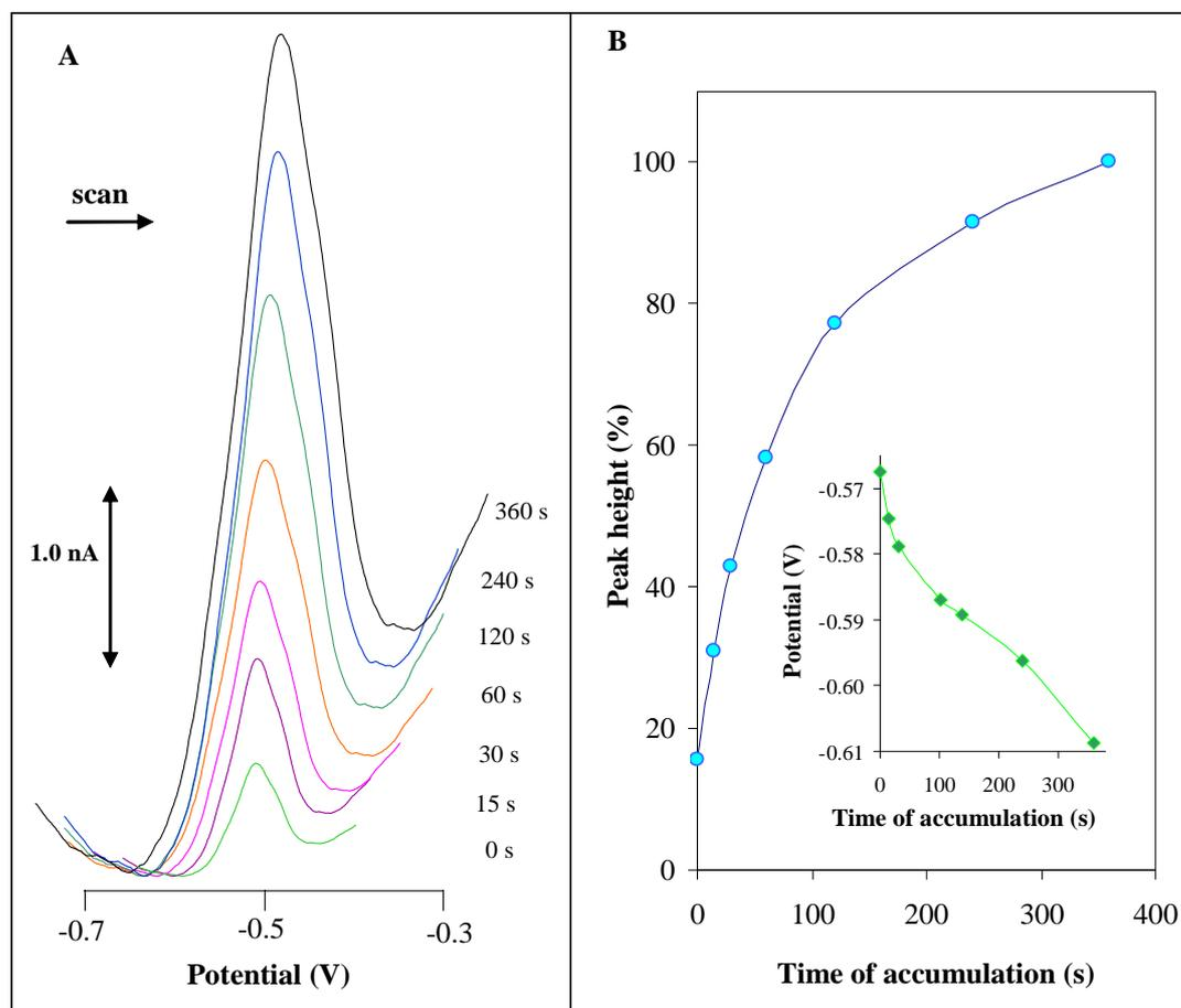
**Figure 5.** Typical DP voltammograms of urease (500 µg/ml) measured under various accumulation times (A). Dependences of urease peak height and its potential (**in inset**) on accumulation time (B). For other details see in Figure 4.
