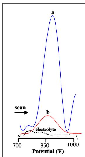
**Figure 8.** Square wave voltammetric analysis of urease using Ni nanoelectrode. The supporting electrolyte (acetate buffer pH 4.2) – dot-and-dash black curve, a) denatured urease (30 min, 99 °C), b) native urease. Concentration of urease (100 mg/ml). SWV parameters were as follows: frequency 200 Hz, initial potential  $-0.4$  V, end potential 1.4 V, step potential 5 mV, amplitude 25 mV.
