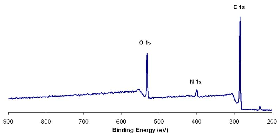
**Figure 6.** XPS survey spectra showing the data gathered for the PANI/PVB/PS3 composite film over the full range of binding energies investigated.
