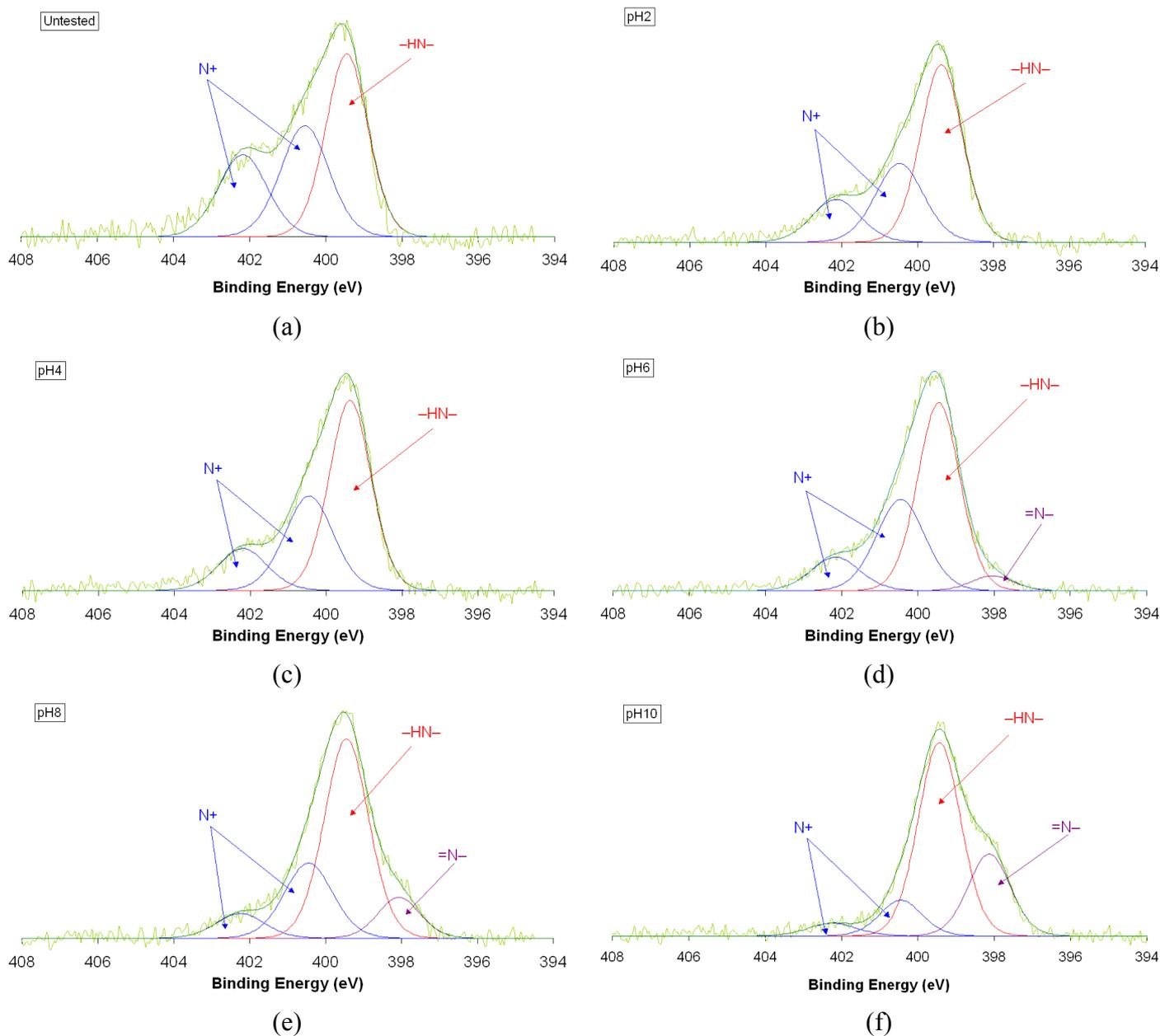
**Figure 7.** XPS spectra (N 1s) of 120 μm PANI composite thick films tested over 96 hours showing: (a) untested film; (b) film soaked in pH2 buffer; (c) film soaked in pH4 buffer; (d) film soaked in pH6 buffer; (e) film soaked in pH8 buffer; and (f) film soaked in pH10 buffer.
