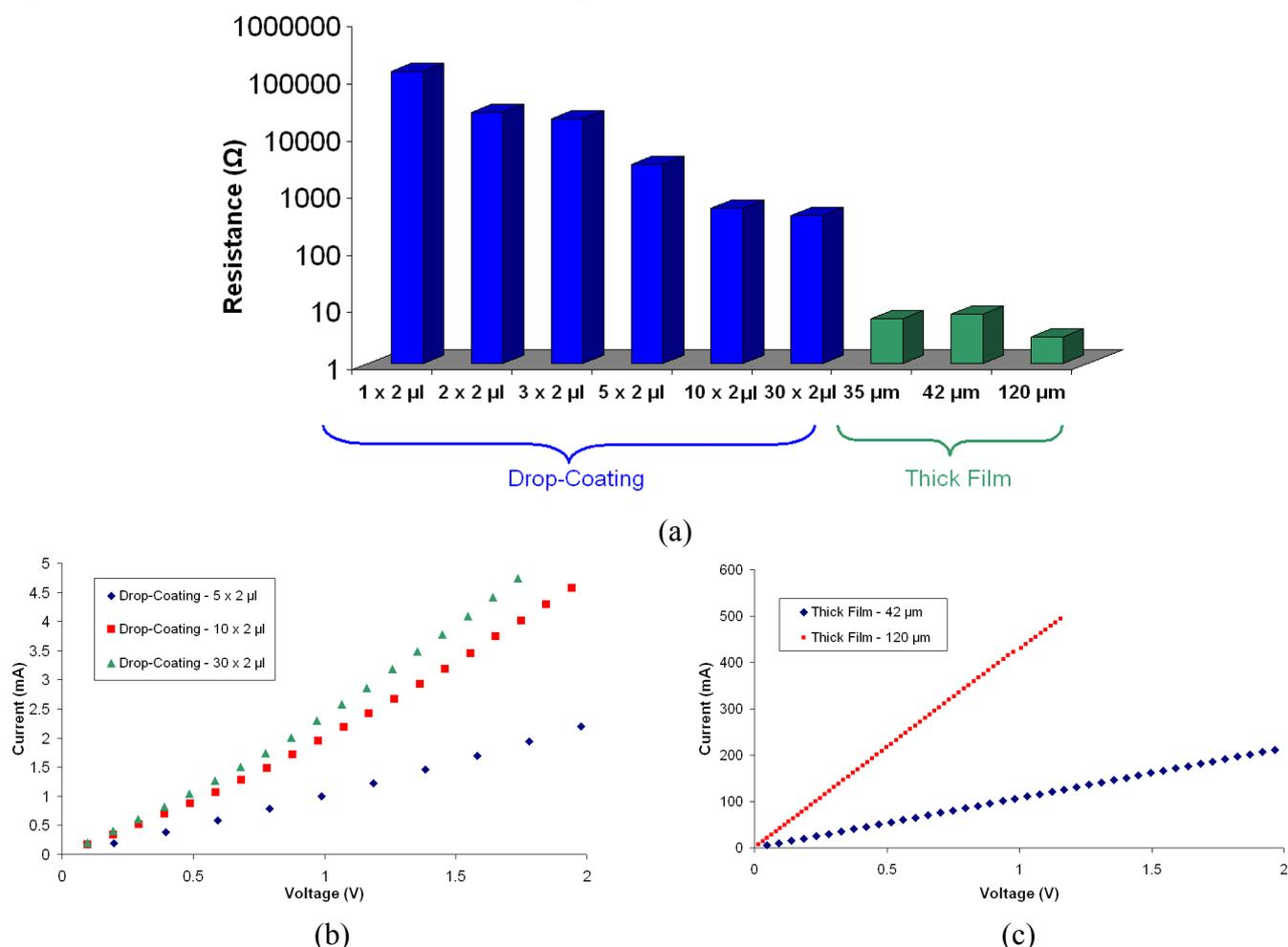
**Figure 3.** DC electrical characteristics of the various PANI films produced using both drop-coating and thick film deposition, showing: (a) the variation of resistance with deposition method; (b) the current-voltage relationship of the Drop-Coated films; and (c) the current-voltage relationship of the Thick films.
