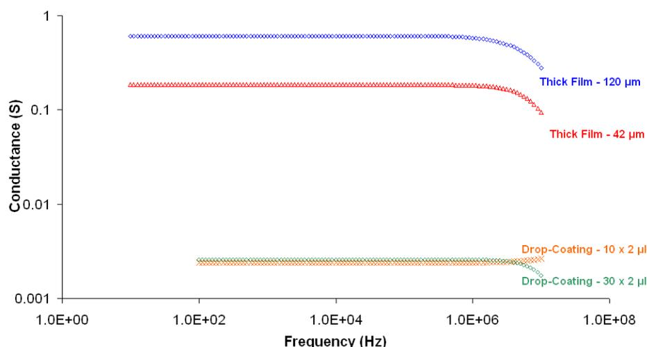
**Figure 4.** AC electrical characteristics of the various PANI films produced using both drop-coating and thick film deposition, showing conductance values taken over a frequency range of 10 Hz to 10 MHz.
