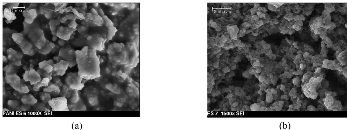
**Figure 8.** SEM micrographs showing: (a) drop-coated (30 x 2  $\mu$ l) PANI/PVB/PS3 composite film; and (b) Screen-printed 120  $\mu$ m thick PANI/PVB/PS3 composite film.
