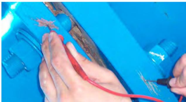
**Figure 5.** Electrical insulation test.
