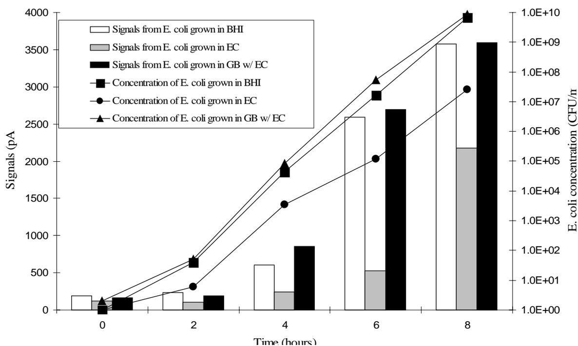
**Figure 4.** Detection of *E. coli* O157:H7 grown in BHI, EC and ground beef (GB) suspended in EC broth in 2 h intervals by using fiber optic biosensor. Bars represent the signals (left X axis) from the biosensor. Lines (growth curves) represent concentrations (right X axis) of *E. coli* O157:H7 grown in broths and ground beef.
