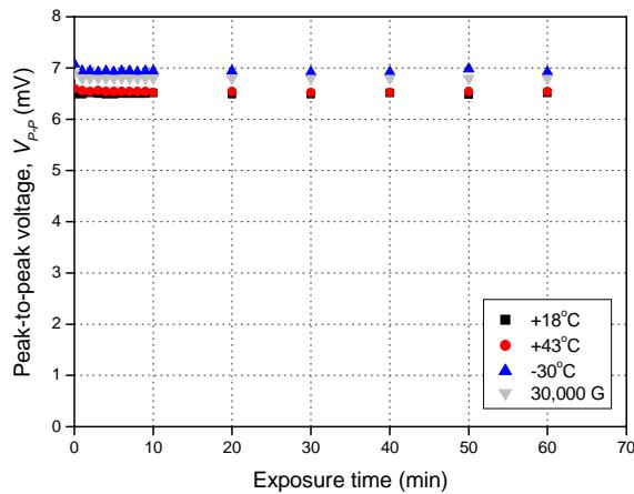
**Figure 15.** Measured drifts of fabricated MMIS at magnetic flux density of 0.05 mT and frequency of 500 Hz.
