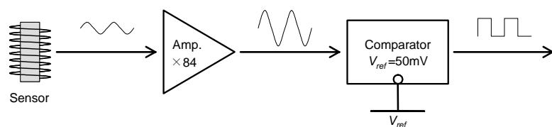
**Figure 3.** Block diagram of signal-processor in turn-counting fuze.
