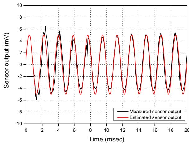
**Figure 17.** Recorded and estimated sensor output signals in firing test.
