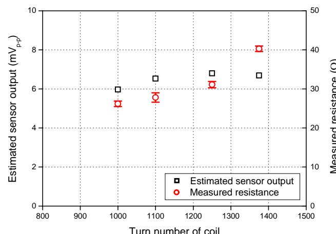
**Figure 6.** Estimated induction voltage of MMIS and measured resistance as function of turn number of coil at magnetic flux density of 0.05 mT, rotational velocity of 30,000 rpm and angle between magnetic field and ammunition rotation axis of 90°.
