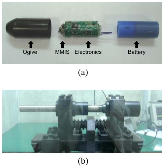
**Figure 16.** Experimental setup for MMIS firing test: (a) Sample projectile with MMIS; (b) Prototype rifled gun.
