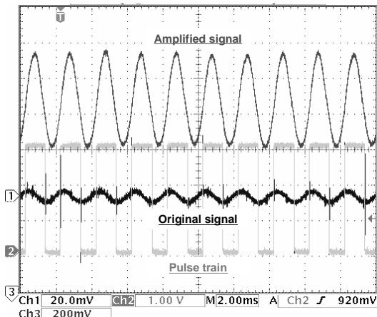
**Figure 12.** Measured sensor signals in signal-processor, where Ch1, Ch2 and Ch3 denote original signal, amplified signal and pulse train, respectively.
