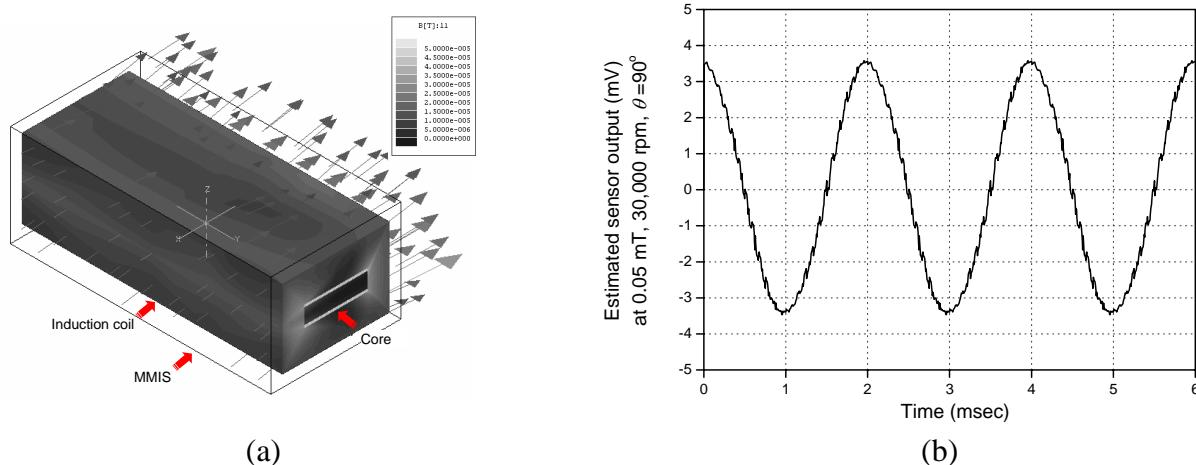
**Figure 7.** Simulation results of MMIS at magnetic flux density of 0.05 mT, rotational velocity of 30,000 rpm and angle between magnetic field and ammunition rotation axis of 90°: (a) Estimated magnetic flux density distribution; (b) Estimated induction voltage of MMIS as function of time.
