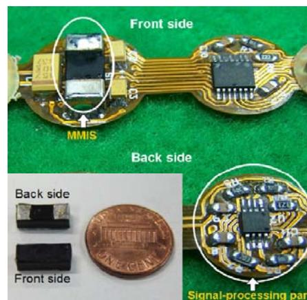
**Figure 8.** Photograph of MMIS and signal-processing part in turn-counting fuze.
