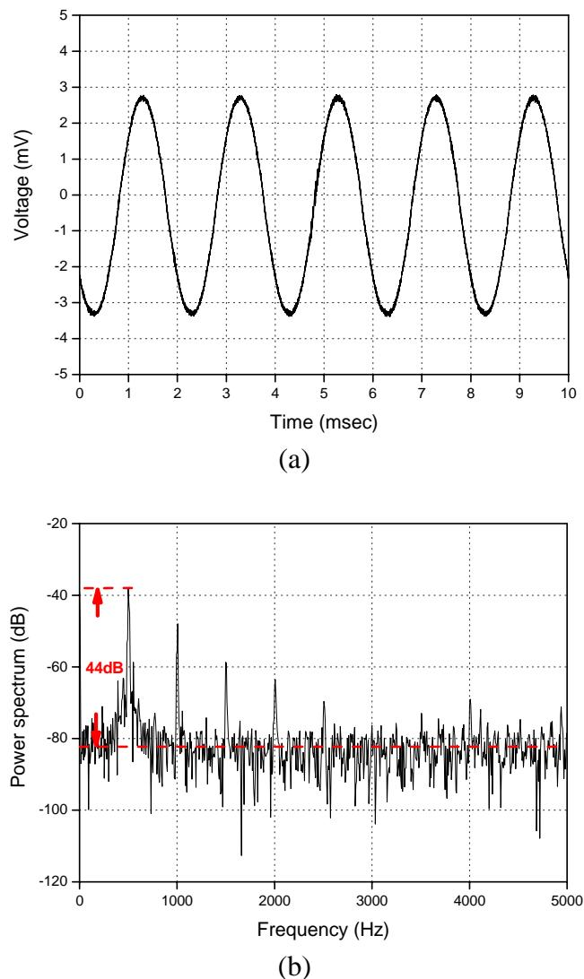
**Figure 10.** Measured sensor output signal of fabricated MMIS at magnetic flux density of 0.05 mT, frequency of 500 Hz and angle between magnetic field and ammunition rotation axis of 90°: (a) Voltage output; (b) Power spectrum output.
