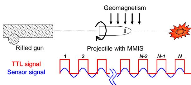
**Figure 4.** Working principle of turn-counting fuze with MMIS.
