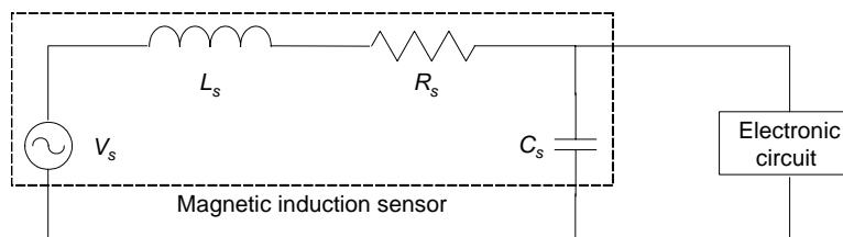
**Figure 5.** Equivalent circuit of MMIS.
