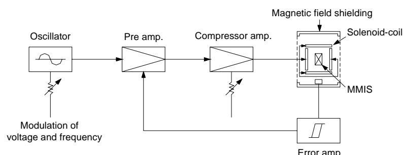
**Figure 9.** Experimental apparatus for static characterization of fabricated MMIS.
