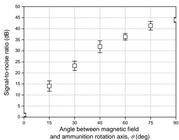
**Figure 11.** Measured SNR of MMIS as function of angle between magnetic field and ammunition rotation axis.
