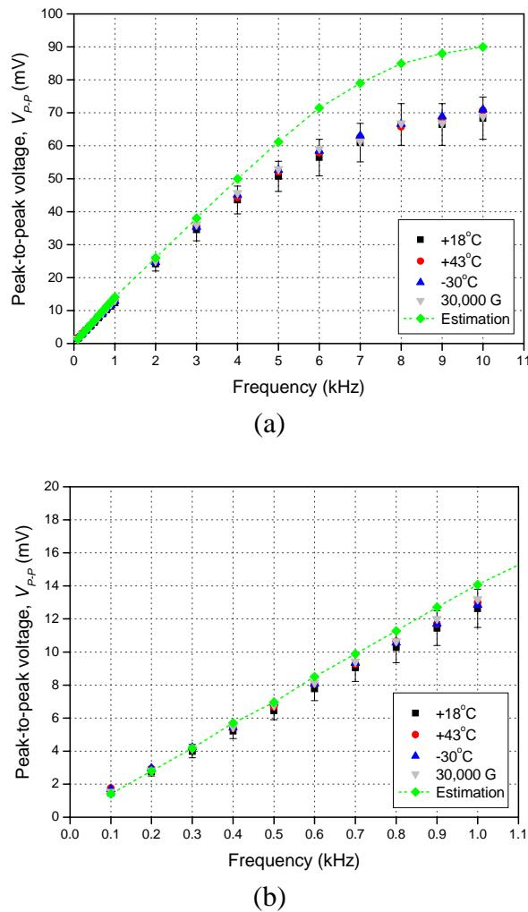
**Figure 14.** Measured and estimated output signals as function of rotational velocity in frequency bands of: (a) 0~10 kHz; (b) 0~1 kHz.
