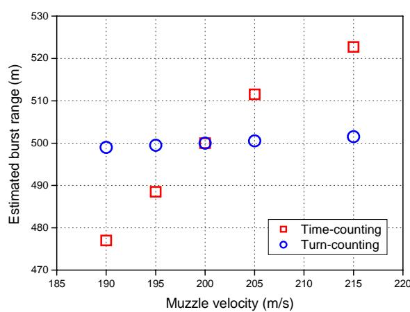
**Figure 1.** Comparison between estimated burst ranges of time-counting and turn-counting fuzes as function of muzzle velocity deviation using simulation results of PRODAS®, where nominal muzzle velocity and nominal burst range are assumed as 200 m/s and 500 m, respectively.
