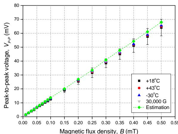
**Figure 13.** Measured and estimated output signals as function of magnetic flux density.
