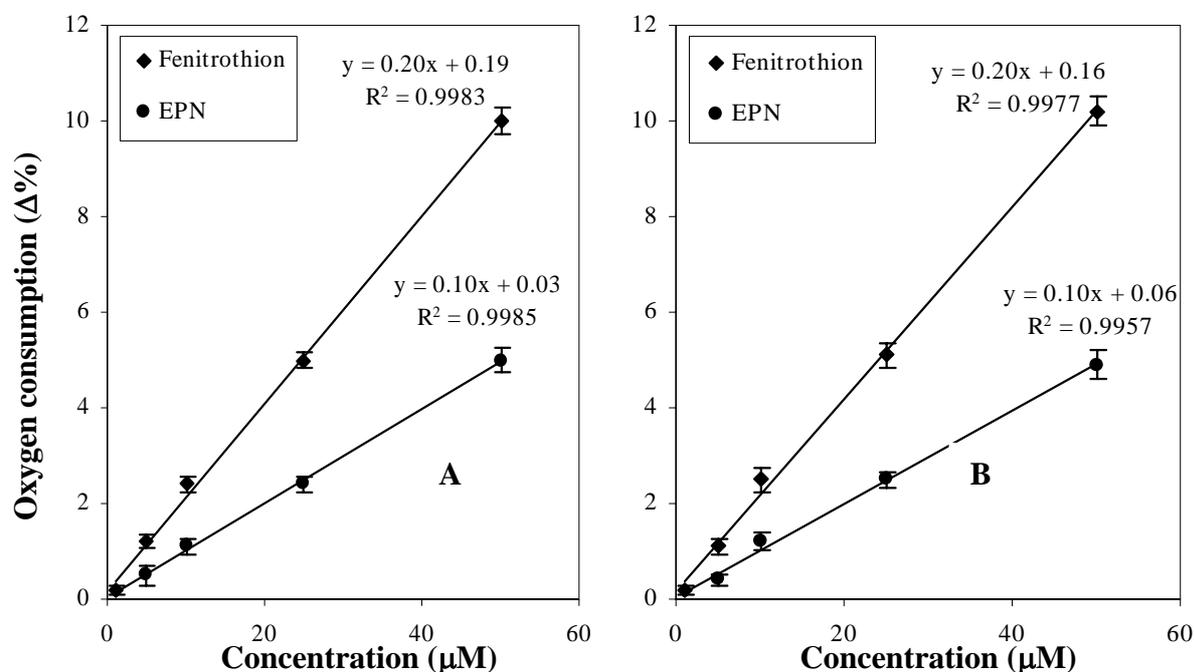
**Figure 1.** Calibration plots for fenitrothion and EPN. A) in 50 mM pH 7.5 citrate-phosphate buffer with 50  $\mu\text{M}$   $\text{CoCl}_2$  and B) in Lake Elsinore water filtered and adjusted to pH 7.5 and 50  $\mu\text{M}$   $\text{CoCl}_2$ , at room temperature, with 0.086 mg cell loading. Data are given as mean  $\pm$  1 standard deviation for three experiments.
