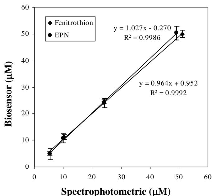
**Figure 2.** Accuracy of microbial biosensor. Fenitrothion and EPN as target compounds and operating in 50 mM pH 7.5 citrate-phosphate buffer with 50 µM CoCl<sub>2</sub> at room temperature, with 0.086 mg cell loading. Data are given as mean ± 1 standard deviation for three experiments.
