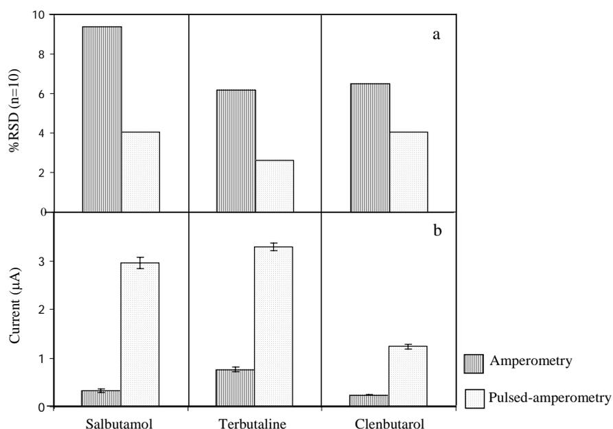
**Figure 5.** Significant improvement in both precision (a) and signal size (b) upon employment of pulsed amperometry with BDD electrode. Results were from replicate injections of salbutamol, terbutaline and clenbuterol standards ( $1 \times 10^2 \mu\text{M}$ ), using the FI system in Fig. 2.
