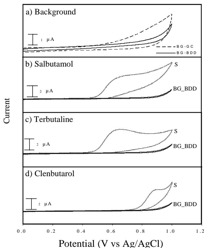
**Figure 3.** Background (BG) and signal (S) voltammograms obtained from 1 mM standard solutions of salbutamol, terbutaline and clenbuterol. Working electrode: BDD or GC. Auxiliary electrode: Pt. Buffer: 50 mM Tris buffer pH 8.3. Scan rate was 100 mV/s.
