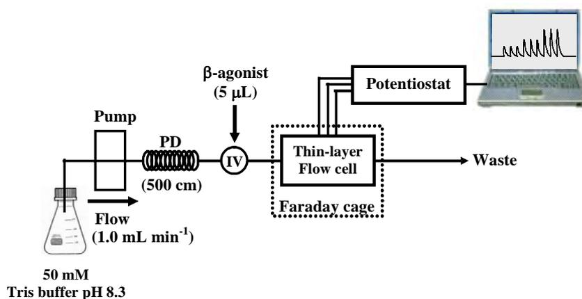
**Figure 2.** The flow injection manifold used in all amperometric measurements, including pulsed amperometry. PD: pulse dampener. IV: injection valve. The condition depicted is optimal configuration with Ag/AgCl and Pt as the reference and the auxiliary electrodes, respectively.
