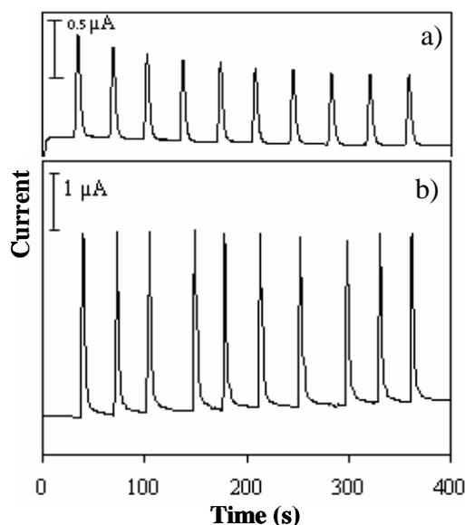
**Figure 4.** Examples of fouling (a) and anti-fouling (b) of BDD electrode for FI detection. Results were obtained from replicate injections of standard salbutamol  $1 \times 10^{-5}$  M to the FI manifold in Fig. 2. (a) amperometric FI with detection potential fixed at 0.6 V. (b) pulsed amperometric FI with the optimized condition shown in Table 1.
