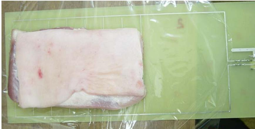
**Figure 34.** Experimental setup for estimation of fat content in pork belly cuts.
