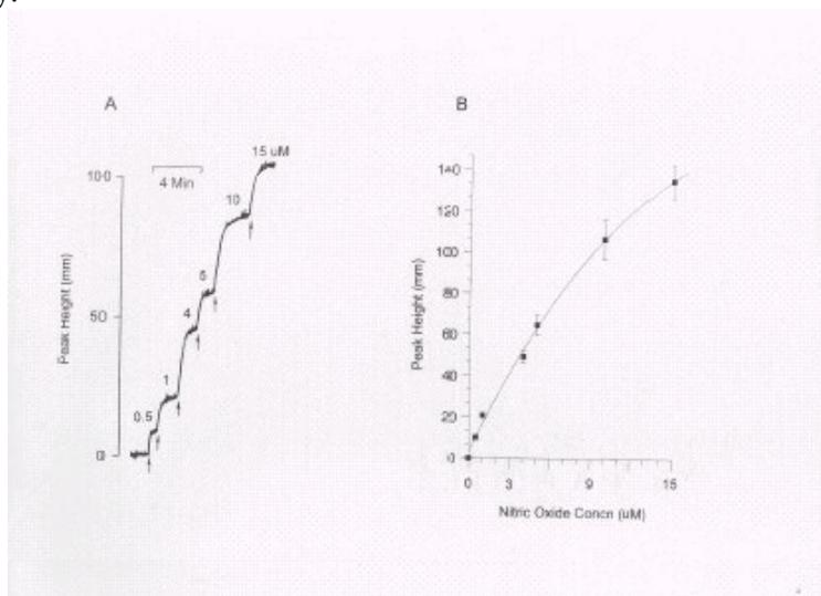
**Figure 1. NO Sensor Calibration.** A: A representative calibration trace showing the responses of the electrode after successive injections (arrows) of  $\text{NaNO}_2$  substrate. B: NO calibration curve generated from 5 separate calibrations. Data are mean  $\pm$  S.E.M. values.
