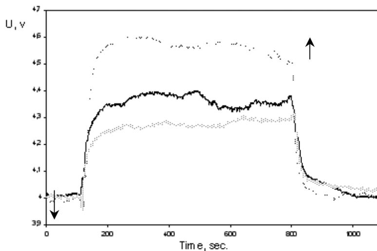
**Figure. 2** Sensor response for 50 ppb of ozone in the air, when Teflon tubes of various lengths are used: 1 cm (upper curve), 500 cm (middle curve), 1000 cm (bottom curve). ↓ - ozone generator ON, ↑ - ozone generator OFF.
