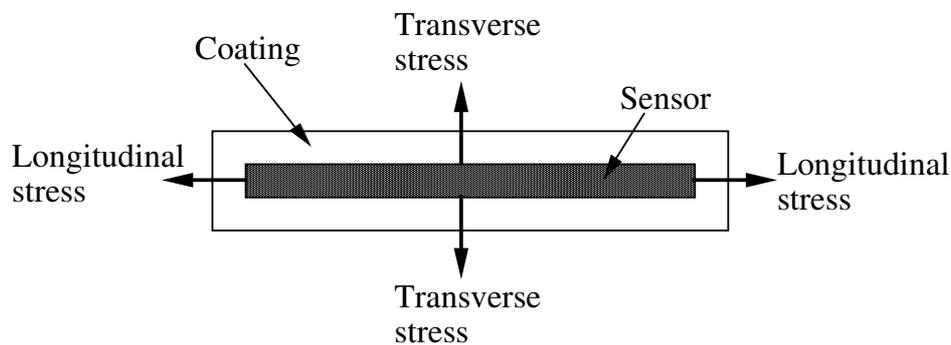
**Figure 2.** Schematic drawing illustrating stresses induced by coating swelling.
