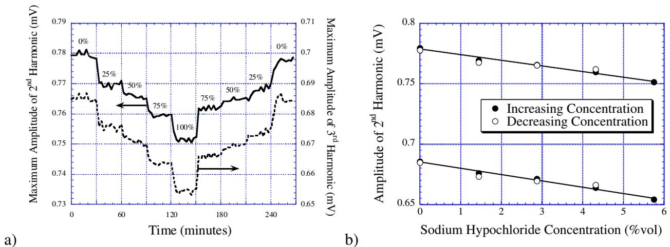
**Figure 6.** (a) The harmonic amplitudes of the sensor when it was exposed to different sodium hypochlorite concentrations. The numbers in the figure are the concentrations of sodium hypochlorite in water. (b) The sensor shows a linear response towards bleach, and the hysteresis between increasing and decreasing concentration is less than 10%.
