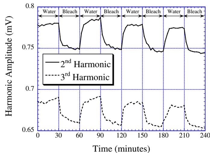
**Figure 5.** The changes in the 2<sup>nd</sup> and 3<sup>rd</sup> harmonic amplitudes when a sensor was cycled between deionized water and 5.75% sodium hypochlorite.
