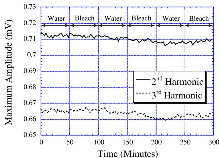
**Figure 8.** The 2<sup>nd</sup> and 3<sup>rd</sup> harmonic amplitudes remained unchanged when a sensor made of Metglas 2714a was cycled between deionized water and 5.75% sodium hypochlorite. This sensor is insensitive to bleach since Metglas 2714a has a low magnetostriction of less than 1 ppm.
