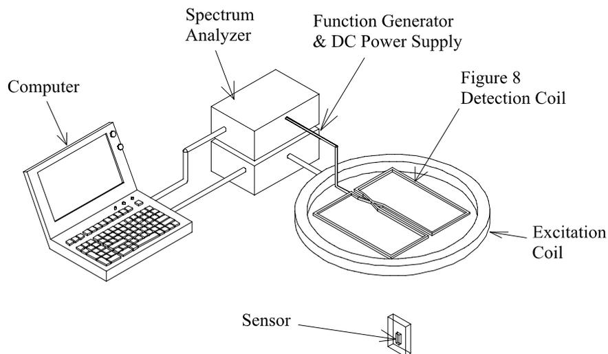
**Figure 1.** Experimental set up for monitoring the harmonic response of a magnetically soft sensor.
