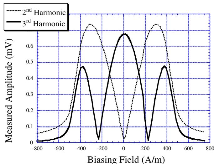
**Figure 3.** The measured amplitude of the 2nd and 3rd harmonics versus amplitude of the dc magnetic biasing field.
