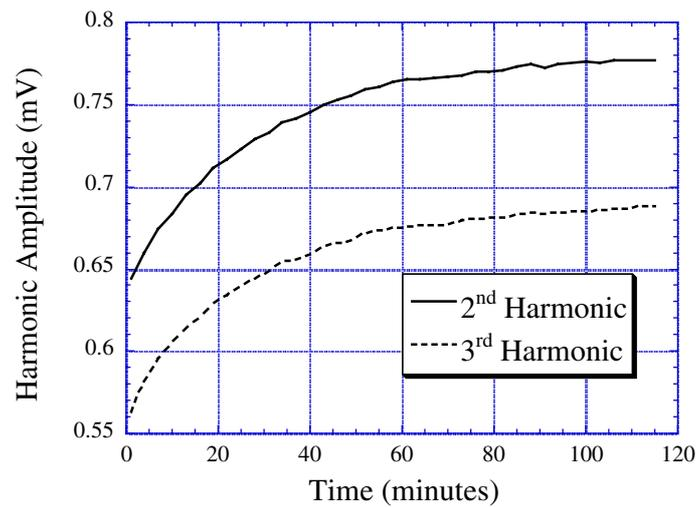
**Figure 4.** Measured variation in the 2<sup>nd</sup> and 3<sup>rd</sup> harmonic amplitudes when a dry sensor was immersed in deionized water.
