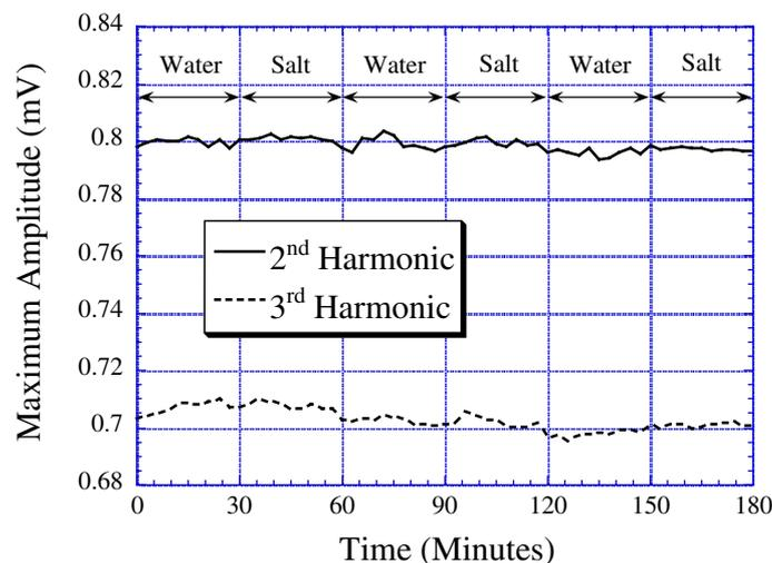
**Figure 7.** The 2<sup>nd</sup> and 3<sup>rd</sup> harmonic amplitudes stayed constant when the sensor was cycled between water and water containing 5.2 g/l sodium chloride (NaCl).
