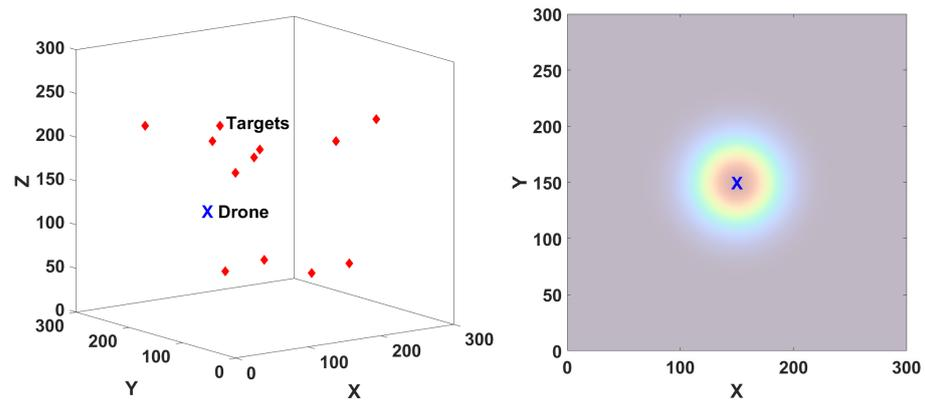
**Figure 1.** Left: 3D space with 12 targets and a drone. Right: drone with a spherical field of view that is symmetrical in all three axes. The dark-orange-to-blue colors show the probability of observation (higher-to-lower) at the current position of the drone. This is a 2D slice of the 3D probability of observation.
