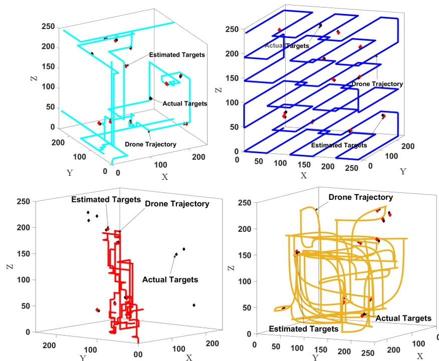
**Figure 6.** Examples of trajectories with the actual targets (black diamonds) and estimated targets (red diamonds). **Top left:** Our method (mutual information with exploration). **Top right:** Lawnmower baseline. **Bottom left:** MI-only baseline adapted from [33]. **Bottom right:** Baseline adapted from [35].
