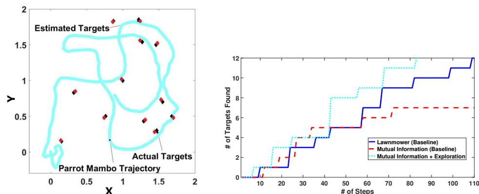
**Figure 14.** Left: Trajectories with our algorithm in 2D real-world with actual and estimated targets. Right: Number of targets detected using real Parrot Mambo minidrone compared to the lawnmower and MI-only baselines.
