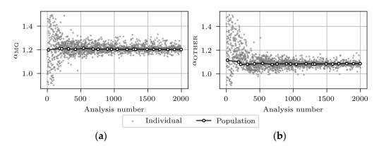
**Figure 17.** Evolution of  $\alpha_{MG}$  (**a**) and  $\alpha_{OTHER}$  (**b**) for FEMU analysis number 5.
