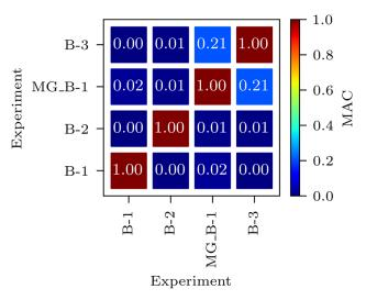
Figure 7. Auto-MAC matrix for the experimental mode shapes.
