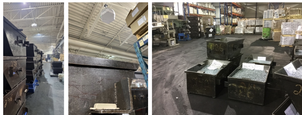
ATR7000 RFID over stacked buckets equipped with tags
