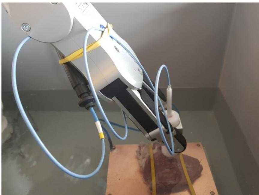
**Figure 3.** A close-up of the experiment, physiological saline solution in the tank and the ex vivo porcine heart on the copper table, during the process of RF ablation.
