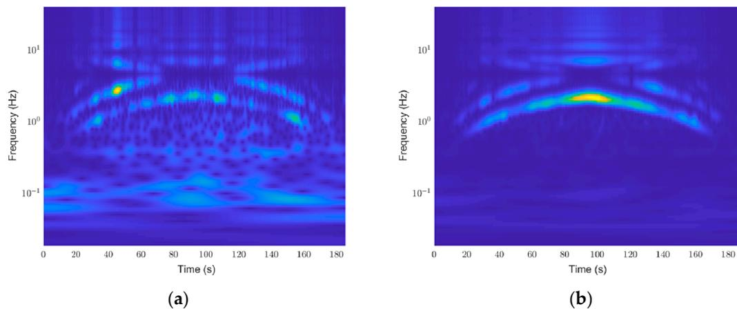
**Figure 5.** Sample scalogram results: (a) Normal (healthy) thruster scalogram; (b) Faulty thruster (breakage; 21% of diameter) scalogram.
