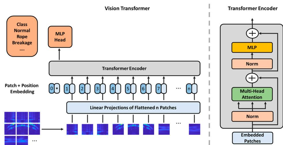
**Figure 6.** The ViT Architecture.
