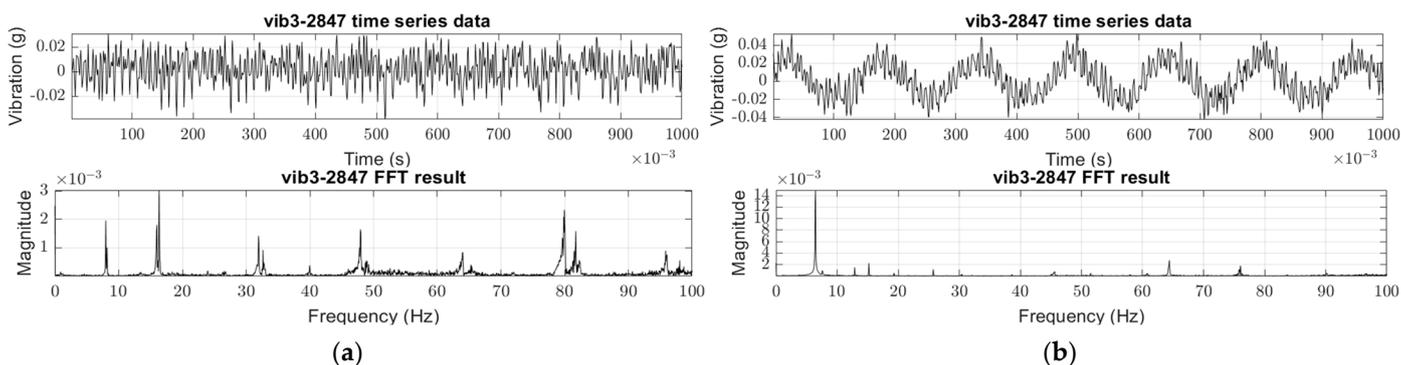
Figure 4. Sample vibration data and its Fast Fourier Transform result (FFT): (a) Normal (healthy) thruster raw vibration and 1X component; (b) Faulty thruster (breakage; 21% of diameter) raw vibration and 1X component.
