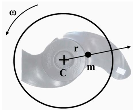
Figure 3. Imbalance on the underwater thruster blade.
