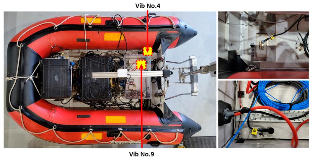
**Figure 14.** Vibration sensor attachment position of both vib No.4 and vib No.9.
