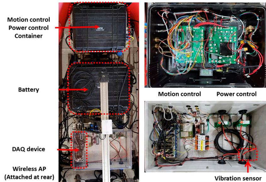
Figure 8. Hardware configuration of FDD USV control systems.
