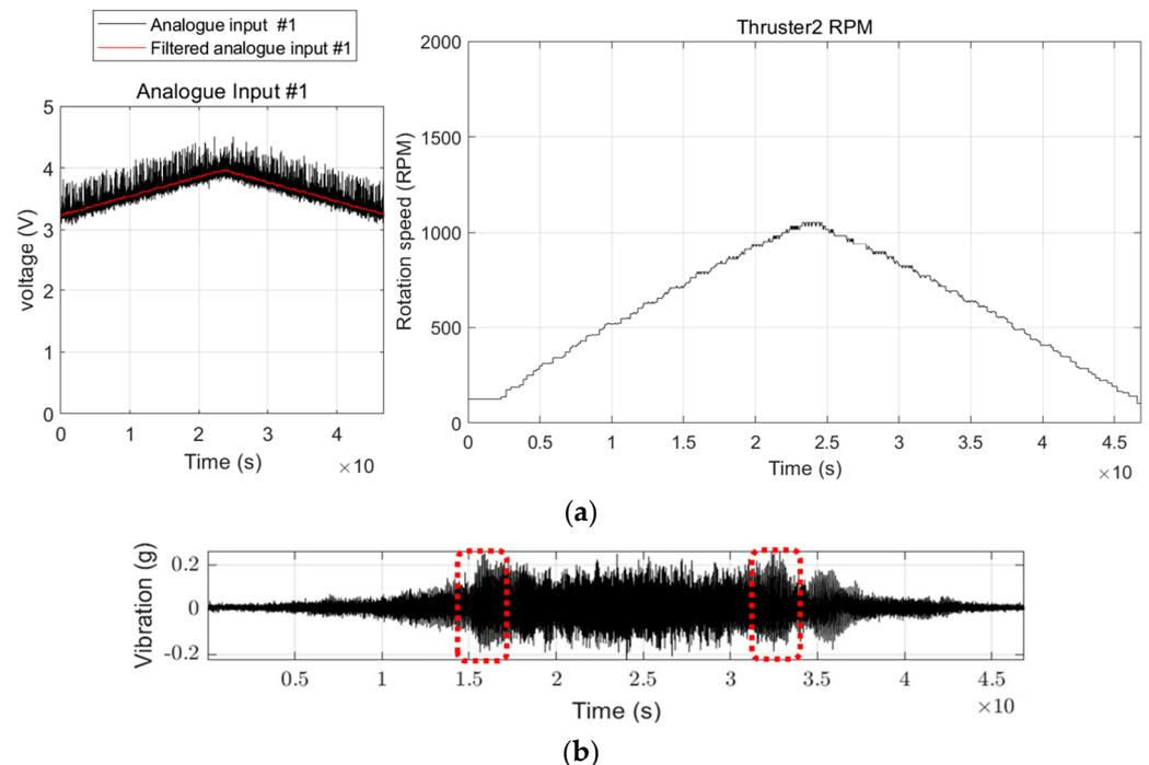
**Figure 7.** Sample data profile of FDD USV: (a) Analogue input, Rotational speed; (b) Acquired vibration data and FDD USV's natural frequency (red dotted square).
