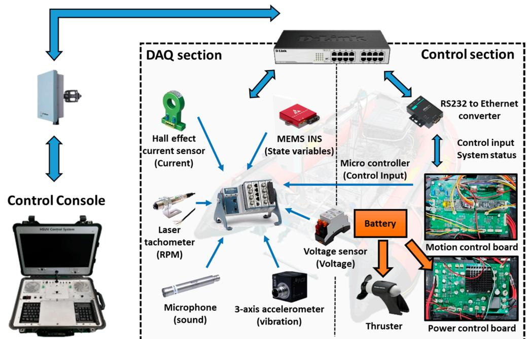
Figure 9. Configuration of FDD USV control and DAQ system.
