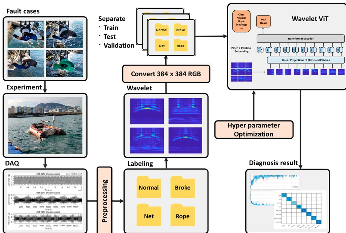
Figure 13. Overall fault diagnosis framework.
