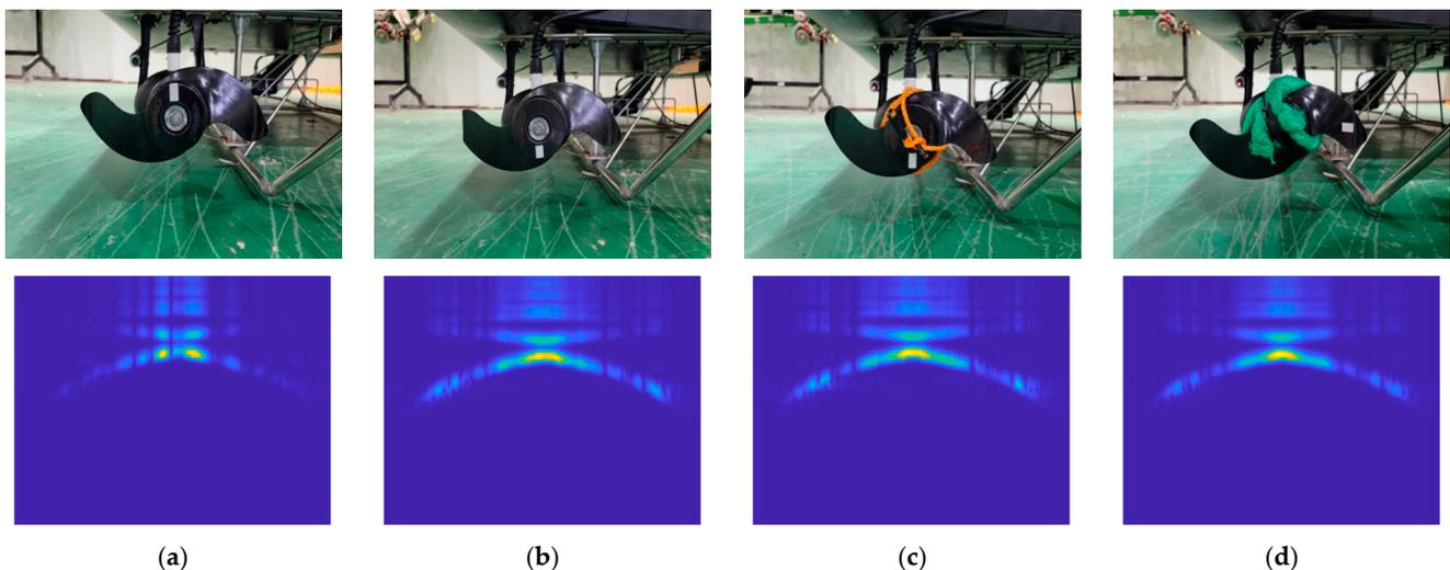
**Figure A1.** On-ground collected fault case and its resulting CWT result: (a) Normal; (b) Breakage 21%; (c) Thin rope entanglement; (d) Net entanglement.
