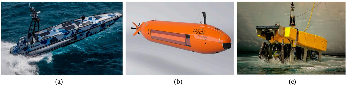
**Figure 1.** Types of unmanned marine platforms: (a) USV; (b) AUV; and (c) ROV.
