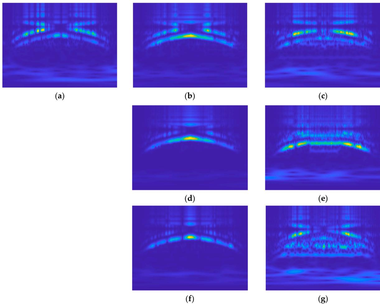
**Figure 11.** Sample result of CWT for test cases: (a) Normal (healthy); (b) Breakage 7%; (c) Thin rope entanglement; (d) Breakage 14%; (e) Rope entanglement; (f) Breakage 21%; (g) Net entanglement.
