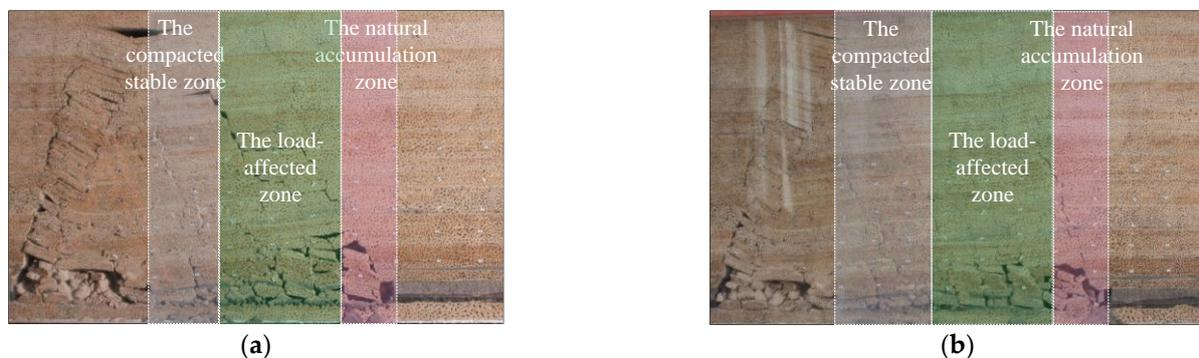
**Figure 8.** Model Excavation Process. (a) The 37th Excavation. (b) The 44th Excavation.
