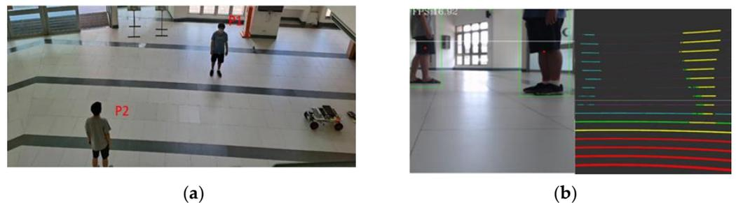
**Figure 19.** (a) Top view of dynamic obstacles in verification field. (b) Integration of LiDAR and imaging in dynamic obstacle detection.
