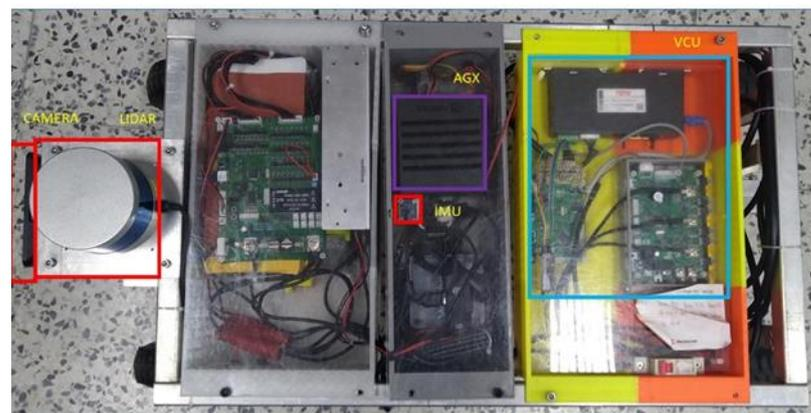
**Figure 3.** Location diagram of related components in Ackerman UMV.
