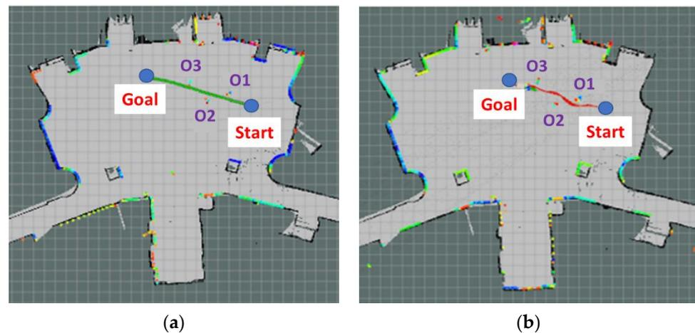
**Figure 17.** (a) Navigation planning path of the system. (b) Moving path of the Ackerman UMV with static obstacles.
