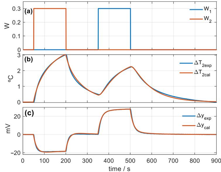
**Figure 2.** Skin calorimeter calibration measurement: (a) powers of the calibration base ( $W_1$  in blue) and of the thermostat ( $W_2$  in red), (b) variation in the thermostat temperature, (c) variation in the calorimetric signal. Experimental curves in blue and calculated in red.
