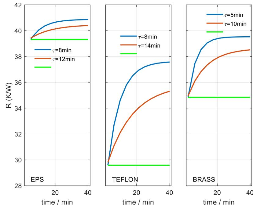
**Figure 9.** Thermal resistance obtained for different materials and as a function of the time considered. Case of invariant hypothesis (red). Variable hypothesis case (Equation (7)): initial value (green) and final value (blue). The figures show the time constant of the exponential fit.
