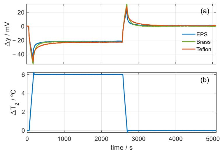
**Figure 6.** Measurements to determine the heat capacity: (a) variation in the calorimetric signal for EPS, brass and Teflon, (b) variation in the thermostat temperature.
