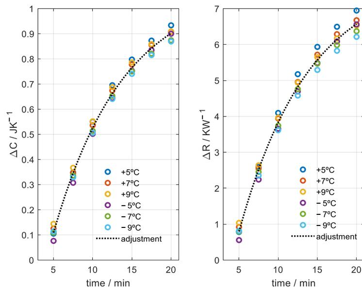
**Figure 11.** Case of Teflon cylinder at the base (see Figure 5). Variation in heat capacity and thermal resistance as a function of time for different temperature changes (+5, +7, +9, −5, −7, −9 °C). Exponential fit (dotted curve with time constant  $\tau = 9$  min).
