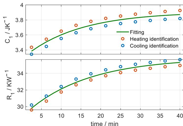
**Figure 7.** Heat capacity ( $C_1$ ) and thermal resistance ( $R_1$ ) as a function of time for the case of applying the calorimeter on a Teflon cylinder. Red dots correspond to the identification of the heating curve and blue dots to the cooling one. The green curve is a fit of all points. The results were obtained under the invariant hypothesis for each time interval considered.
