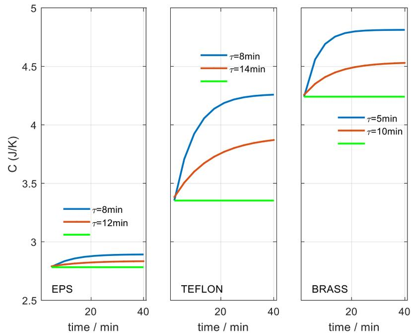
**Figure 8.** Heat capacity obtained for different materials and as a function of the time considered. Case of invariant hypothesis (red). Variant hypothesis case (Equation (7)): initial value (green) and final value (blue). The figures show the time constant of the exponential fit.
