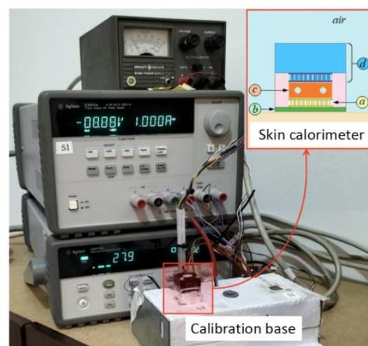
**Figure 1.** Instrumentation and skin calorimeter placed on calibration base. Schematic of the calorimeter: (a) measurement thermopile, (b) aluminum plate, (c) thermostat, (d) cooling system.
