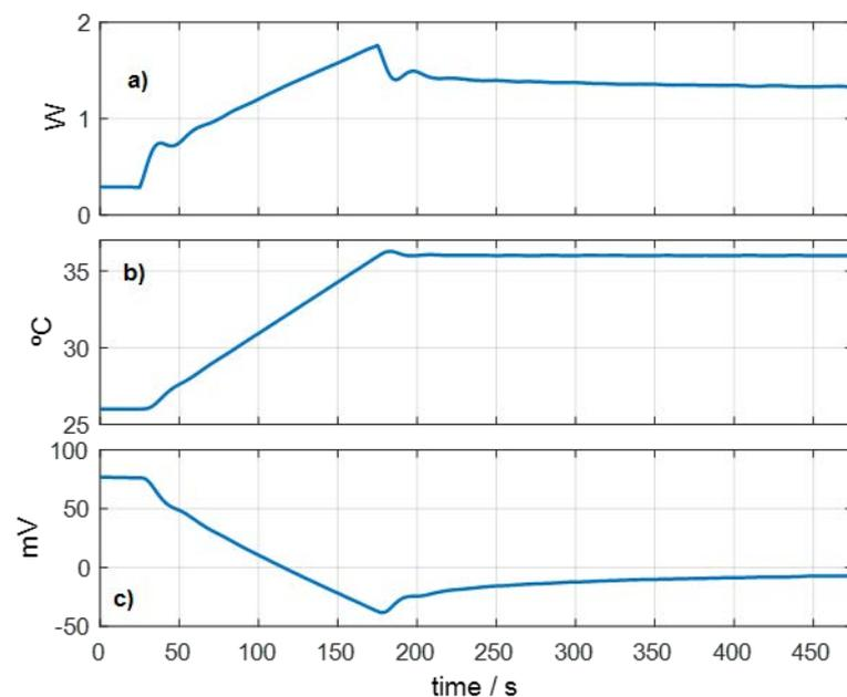
**Figure 4.** Measurement to determine the thermal properties of the skin, performed on the volar area of the right wrist of a healthy 64-year-old male subject. (a) Thermostat power ( $W_2$ ), (b) thermostat temperature ( $T_2$ ), (c) calorimetric signal ( $y$ ),  $T_{room} = 24.1$  °C.
