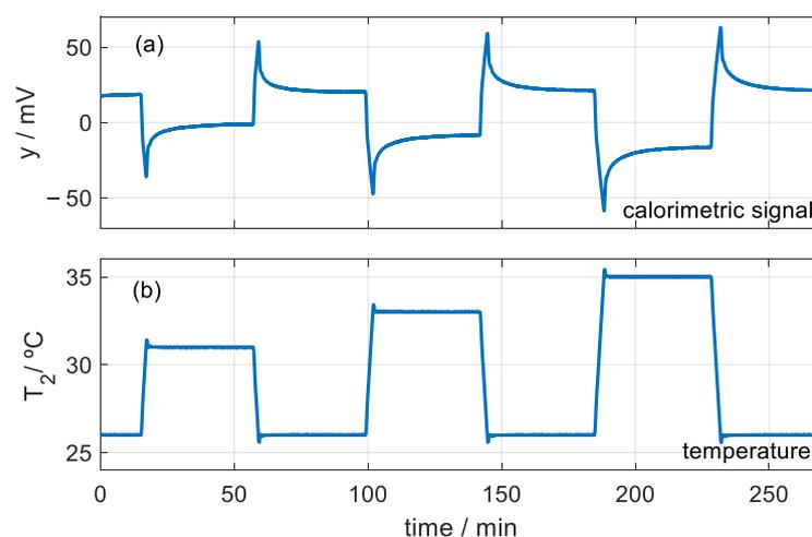
**Figure 10.** Calorimetric signal (a) of an experimental measurement for studying the variation in the heat capacity as a function of the thermostat temperature change (b).
