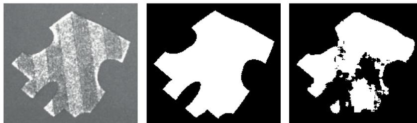
**Figure 14.** Segmentation error of part 4 at height 25.2 mm due to inhomogeneous lighting. Left: Camera image, middle: mask, right: segmentation.
