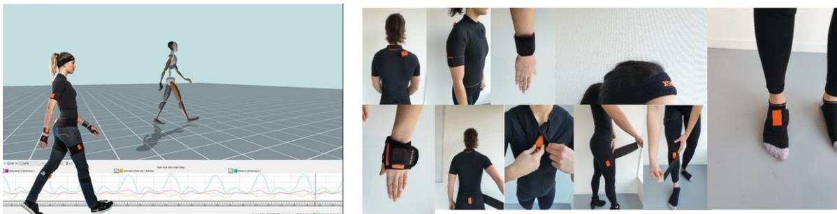
Figure 2. Xsens Awinda inertial motion sensors and its location.
