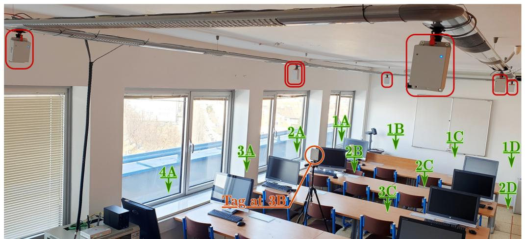
Figure 5. Testbed photography; anchors are highlighted by red rectangles (master anchor by double rectangle); visible test locations marked by green arrows; tag is highlighted by orange circle.
