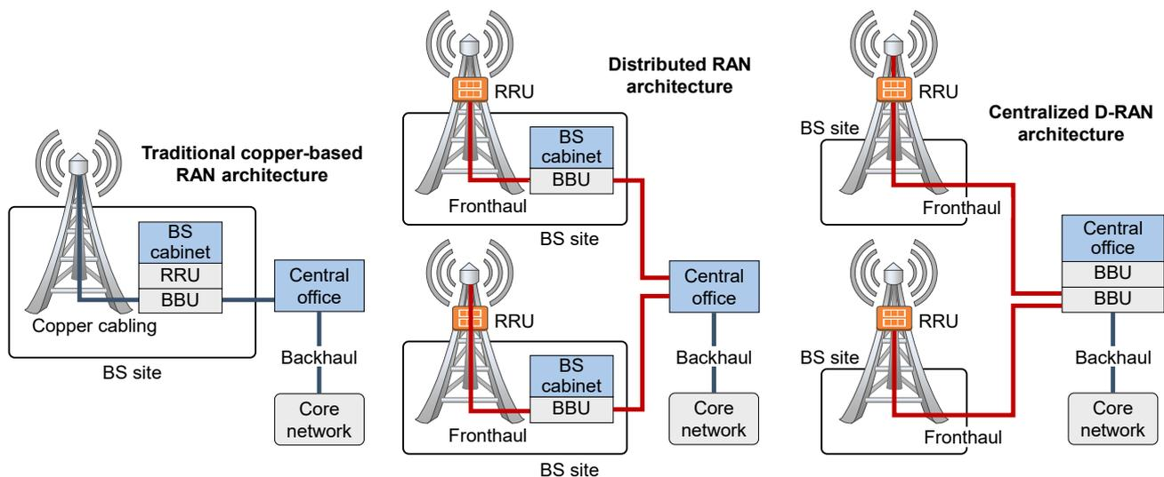
**Figure 1.** Comparison of traditional RAN and D-RAN architecture.
