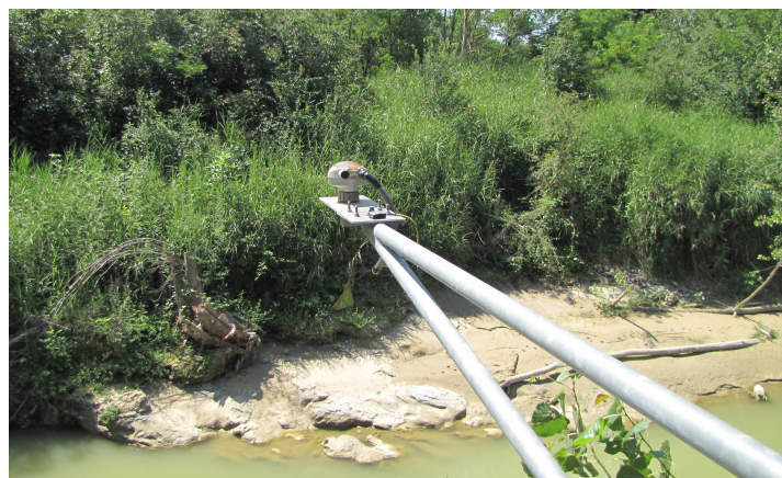
Figure 7. Example of a gauge ultrasonic sensor used to acquire the stages measurements (SITRANS Probe LU, Table 1).
