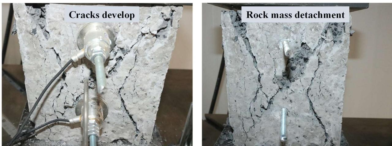
Figure 9. Failure modes of anchor–grouting system specimens.
