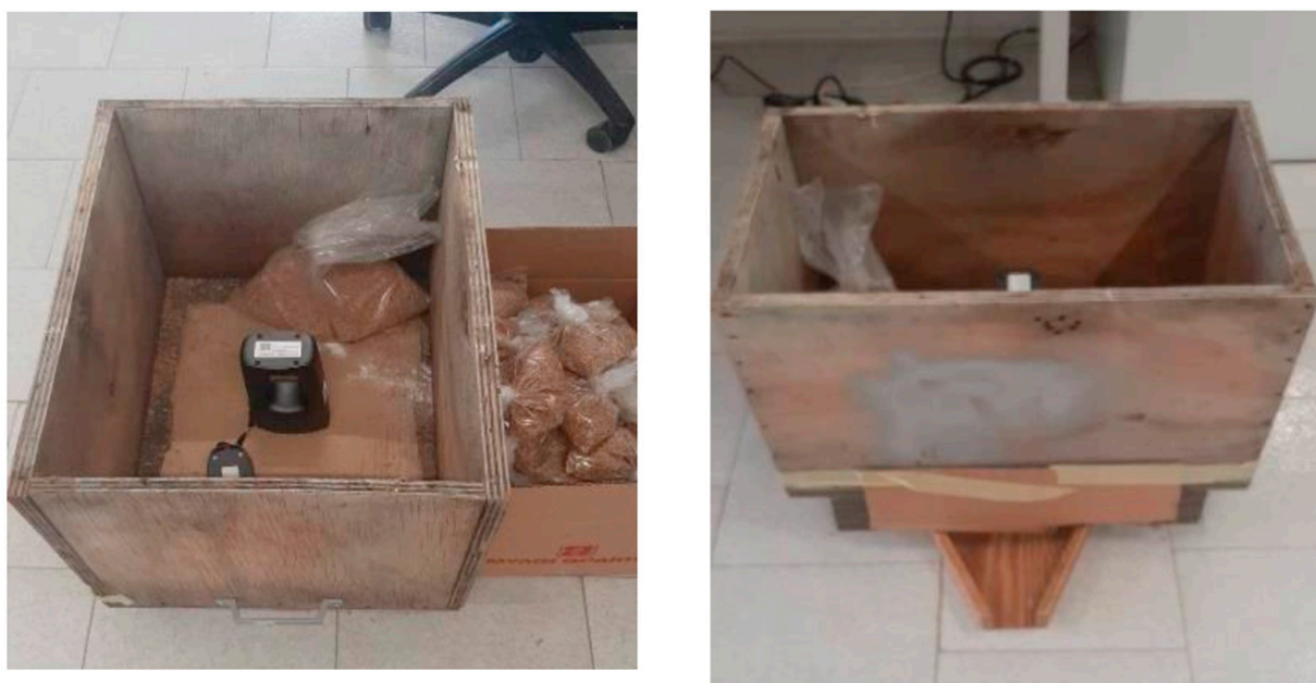
Figure 1. Capturing the spectral profiles of wheat samples within the experimental setup.
