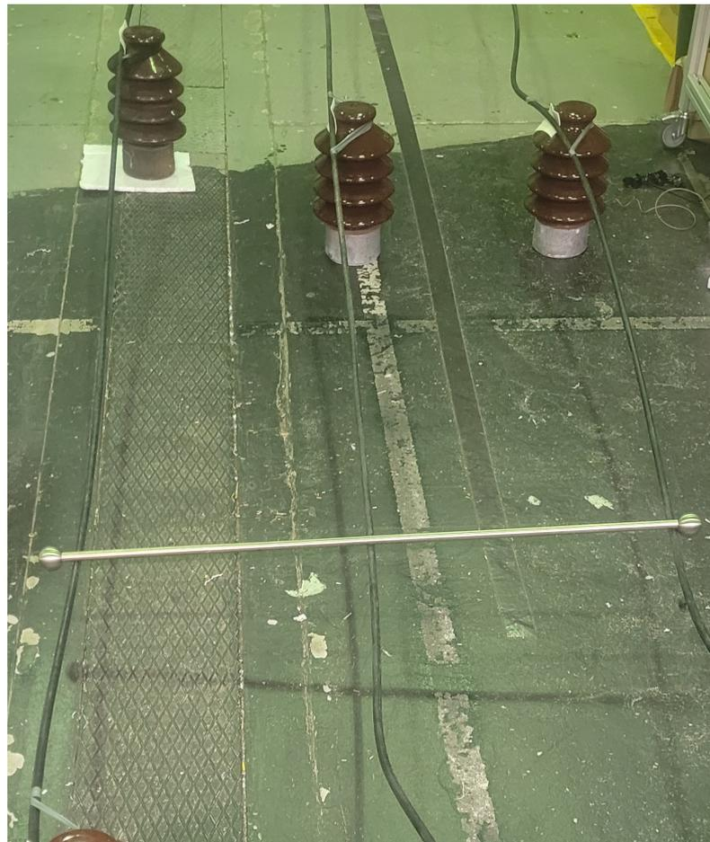
**Figure 4.** Balanced fault between all three phases.
