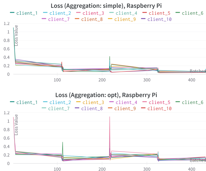
Figure 6. Loss comparison for different federated aggregation techniques using 10 Raspberry Pi devices. The x-axis represents the incremental number of training mini-batches, the y-axis represents loss-values.
