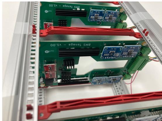
**Figure 8.** Detailed view of the assembly of a designed PCB mounted in the rack.
