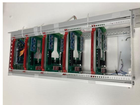
**Figure 7.** Integrated circuit assembly in a rack with the Arduino card. General overview.
