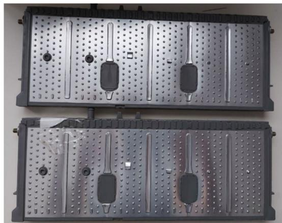
**Figure 9.** Details of two commercial cells tested in this case study: Toyota Prius battery cells.
