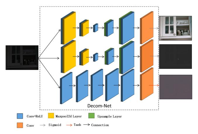
Figure 2. The model structure diagram of the Decom-Net.
