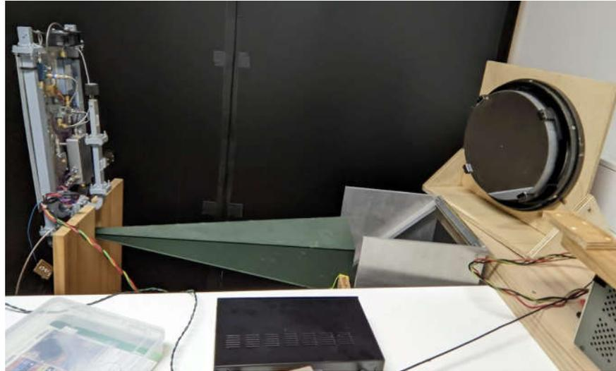
**Figure 14.** The radar signal for the RASS is radiated from the green horn and reflected upwards by a fine-wire grid mounted at  $45^\circ$  to the beam, while the acoustic signal is radiated through the grid and upwards in front of the parabolic mirror. The camera and light source are off the photo on the left and are pointed towards the mirror.
