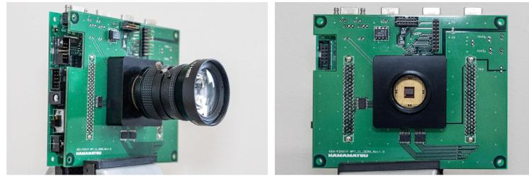
**Figure 9.** Appearance of the prototype camera made by Hamamatsu Photonics K.K. We used this prototype camera to capture the actual scene.
