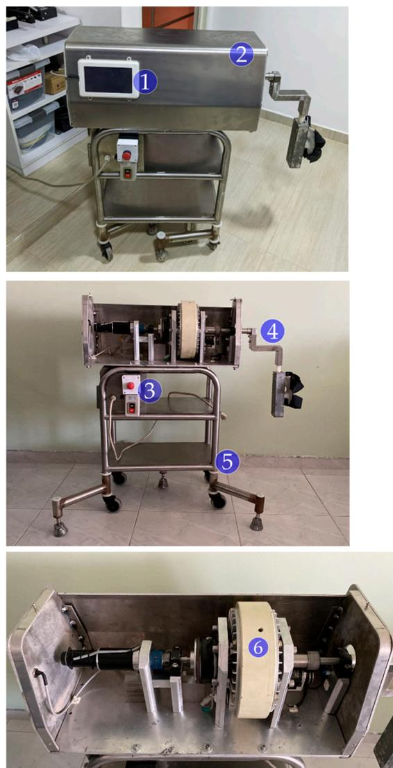
**Figure 1.** Rehabilitation device configured for a lower limb rehabilitation system from Universidad del Valle: (1) control screen; (2) chassis; (3) emergency; (4) foot pedal; (5) support structure stop; and (6) magnetic brake.
