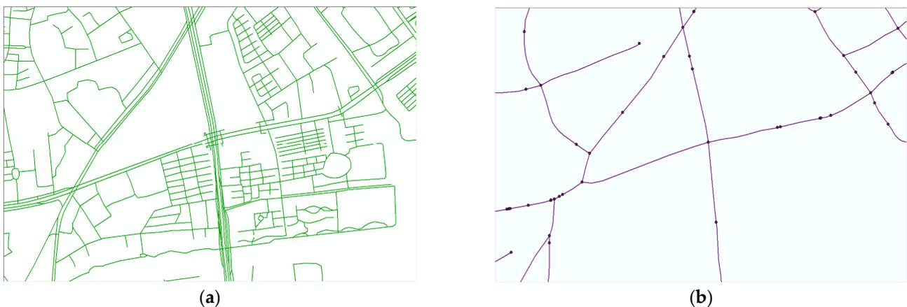
**Figure 2.** The processes of developing a topological map. (a) The original map of an intersection. (b) The final topological map.
