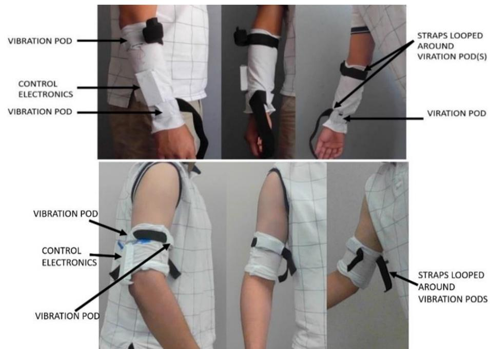
**Figure 4.** Top: Forearm sleeve with straps open. Embedded focal vibration pods and a control electronics box are labeled. These can be removed if the sleeve needs to be washed. Bottom: when the vibration pods and control electronics are attached to the upper arm with the sleeve.
