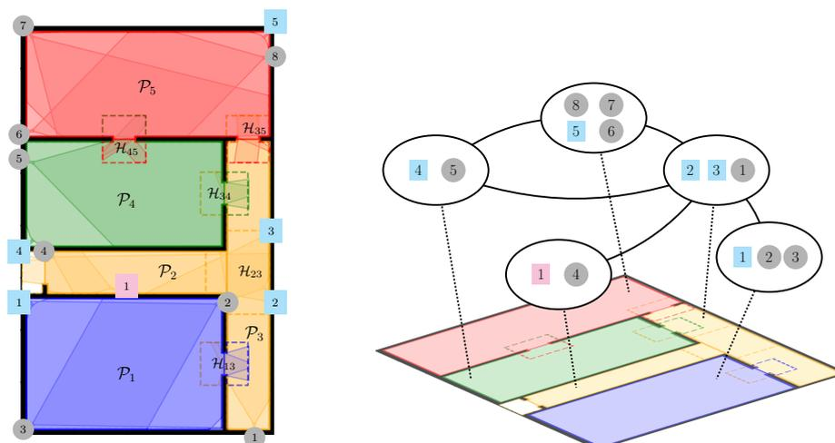
**Figure 1.** Environment example: colors distinguish the physical environment partitions; dashed lines identify the handout zones among virtual environment partitions; cameras are indicated with round and square markers.
