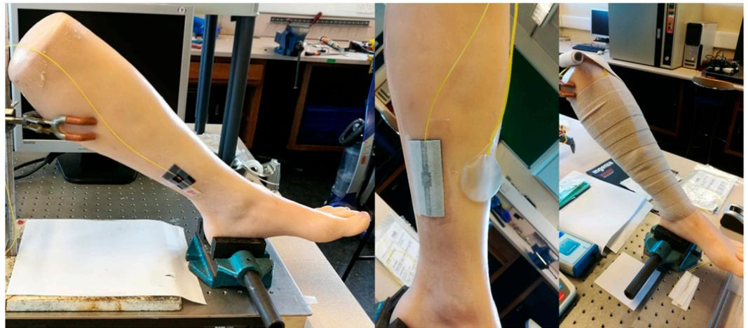
**Figure 5.** Custom-made phantom leg shown with sensors (optical fibre and PicoPress) at the approximate B1 position and with a full bandage wrap.
