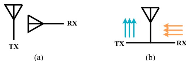
**Figure 6.** Polarization orthogonality realizations in (a) multi-antenna system and (b) single/shared antenna system.
