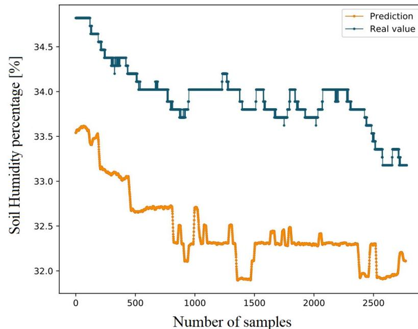
**Figure 5.** Soil moisture estimation using the SVR model on the test set compared to expected soil moisture values [6].
