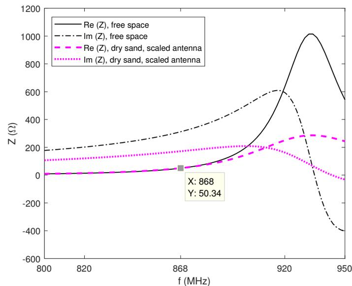
**Figure 8.** Simulation results for antenna impedance in free space and scaled antenna in dry sand.
