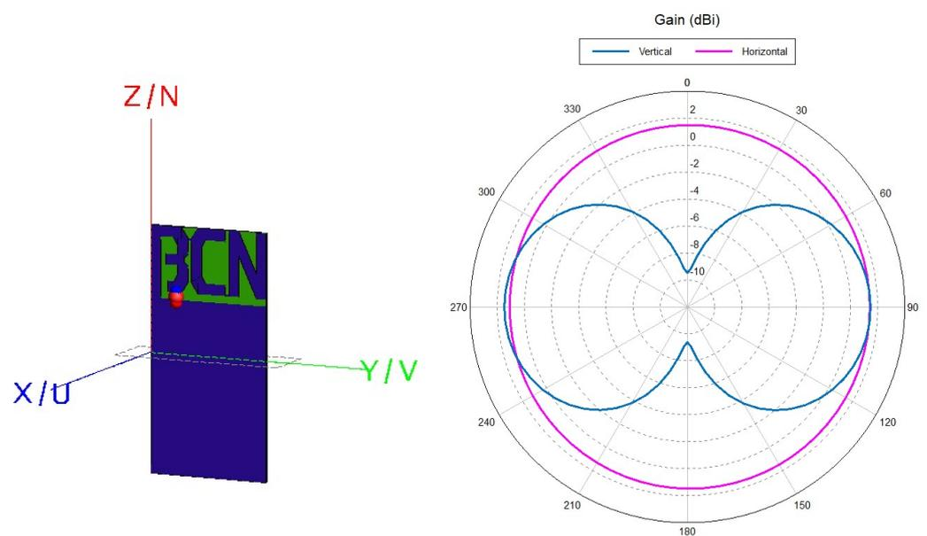
**Figure 7.** Simulation model of PIFA antenna in FEKO and its 2D radiation pattern for gain in dBi at 868 MHz.
