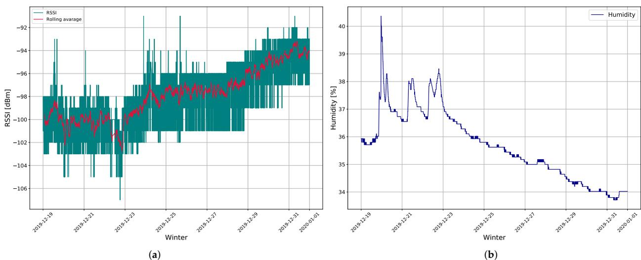
**Figure 3.** The measurement results of: (a) RSSI in dBm collected from gateway 2 and (b) soil moisture during the winter period.
