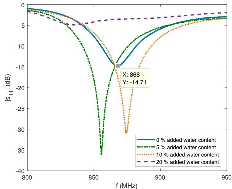
**Figure 12.** Reflection coefficient measurements of antenna buried in sand with four levels of moisture content.
