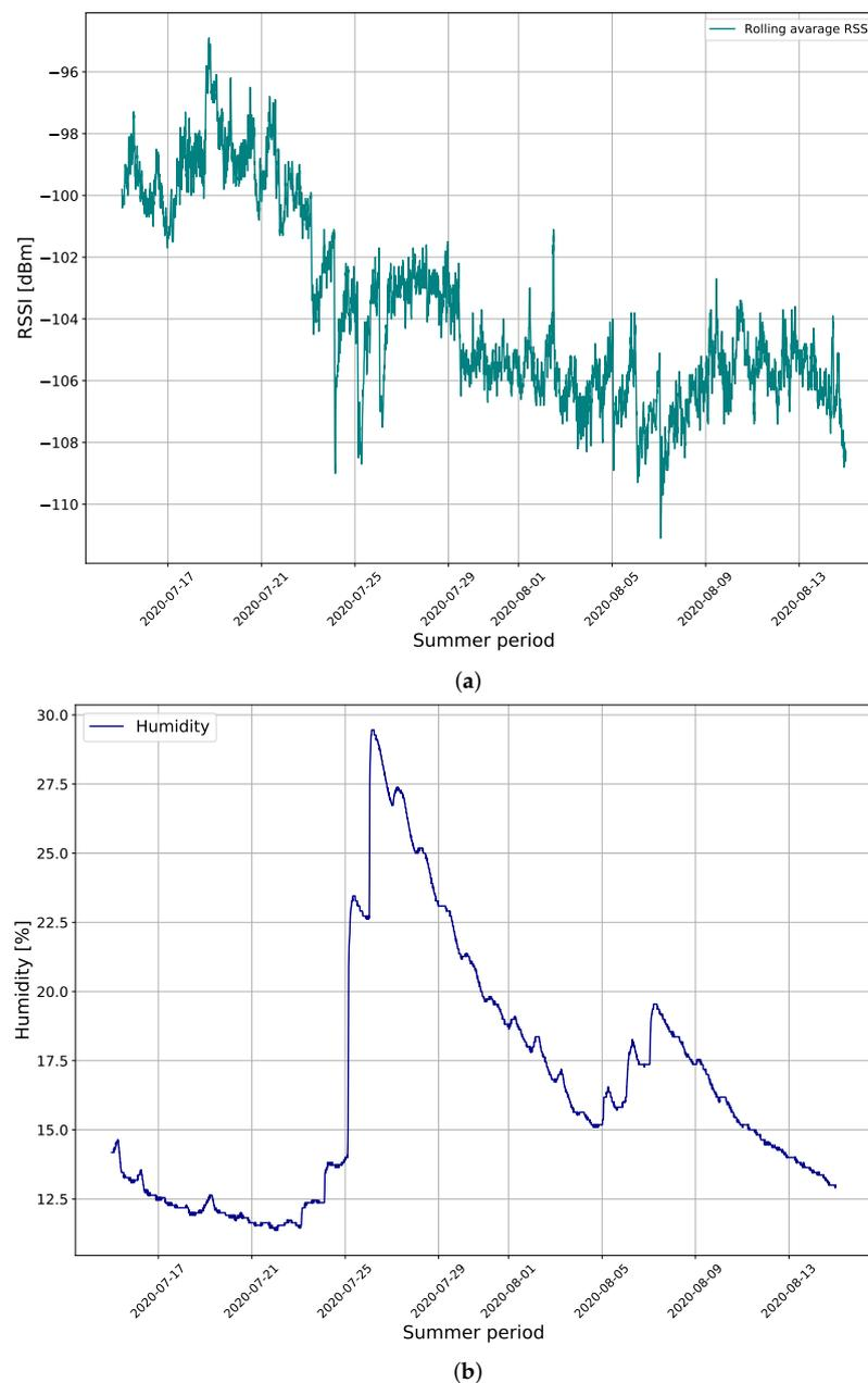
**Figure 6.** The measurement results of: (a) RSSI in dBm collected from gateway 2 and (b) soil moisture during the summer period.
