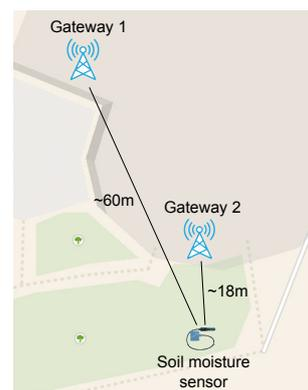
**Figure 2.** Implementation of LoRaWAN-based soil moisture sensing device.
