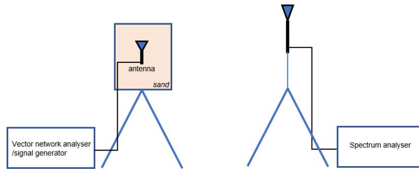
**Figure 11.** Setup for received signal power measurement.
