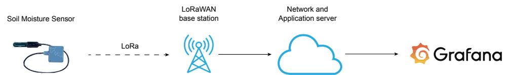
**Figure 1.** Network architecture of LoRaWAN-based soil moisture sensor system.
