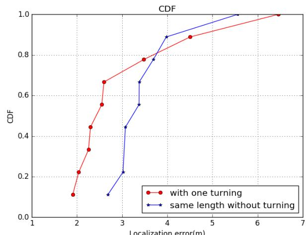
**Figure 11.** Figure shows CDF with localization error. The left curves represent steps with turns, the right denote the track at the same length without any turn. We can see that 80% of the errors occurred in less than 2.5 m.
