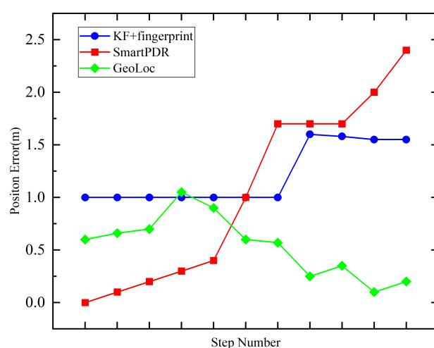
**Figure 22.** Relationships between step number and positioning error using different positioning methods.
