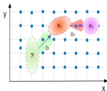
**Figure 3.** Uncertainty eliminates algorithm diagram explanation. From left to right is the user's motion estimation. The colors of the fan-shaped area and circle area denote the uncertainties. In each step, the searching space, acreage in the figure, is diminished.
