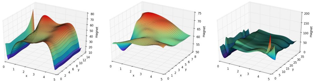
**Figure 19.** Magnetic map near landmarks: lift, vendor machine, and corridor, separately.
