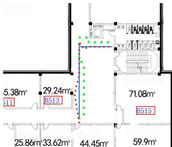
**Figure 18.** Floor plan of 6th floor, with estimation and true trajectories. The triangle line, or the polygonal line, represents normal Kalman-filter-based localization; the straight line with regular turning represents the test walking path, and the line with the red five-pointed star shows the results of GeoLoc.
