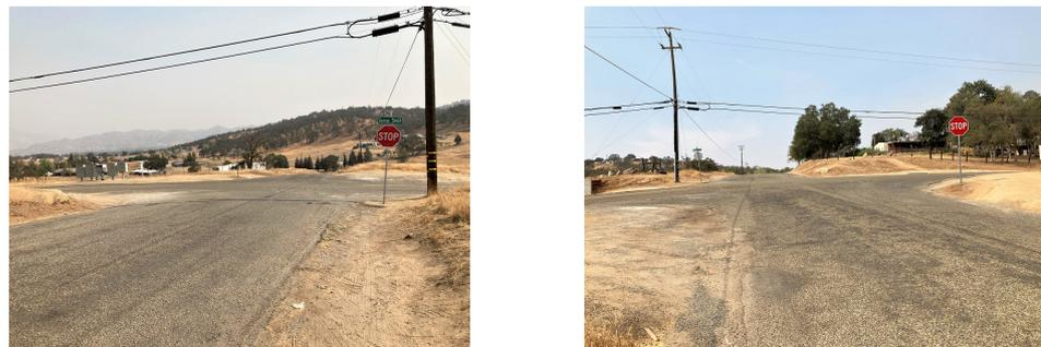
**Figure 5.** Example rural intersection from the point of view of vehicles traveling east–west through the intersection. Note that lack of visibility of traffic approaching in the north and south direction.
