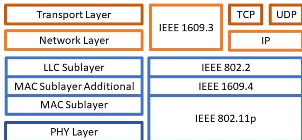
Figure 3. Visual representation of DSRC layers and protocols taken from [15].
