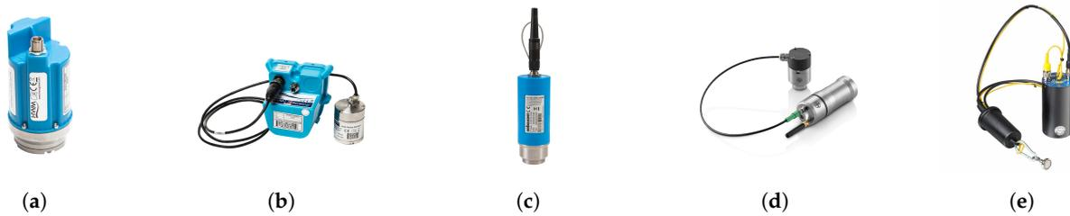
**Figure 1.** Range of vibro-acoustic loggers installed across metropolitan Sydney: (a) HWM PermaNET SU, (b) HWM PermaNET+, (c) SebaKMT Sebalog N-3, (d) Von Roll ORTOMAT-MTC, (e) Primayer Enigma3m.
