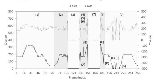
**Figure 7.** Real—time trace of XY coordinates for the bounding box from the vertical low angle: numbers  $(1)\sim(9)$  stand for different statuses; letters (A) and (E) $\sim$ (G) represent detection failure events; letters (B) $\sim$ (D) represent scene change events.
