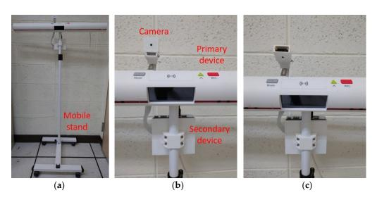
**Figure 2.** System prototype: (a) system with mobile stand; (b) camera capturing a horizontal view; (c) camera capturing a vertical view.
