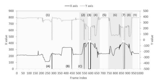
**Figure 6.** Real—time trace of XY coordinates for the bounding box from the horizontal low angle: numbers (1)~(9) stand for different statuses; letters (A)~(C) represent detection failure events.
