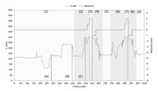
**Figure 9.** Behavior index trace from the horizontal low angle: numbers (1)–(9) stand for different statuses; letters (A)–(C) represent detection failure events.
