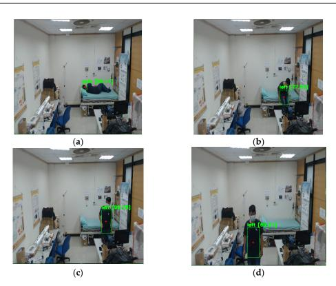
**Figure 8.** Images from the diagonal high angle: (a) lay on the bed; (b) get up and turn around; (c) sit on the edge of bed; (d) exit the bed.
