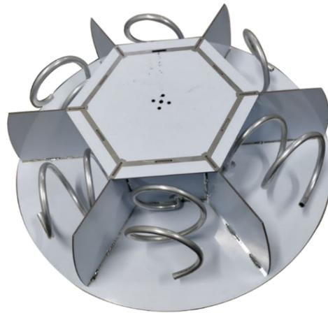
**Figure 8.** Physical picture of directional spiral antenna array.
