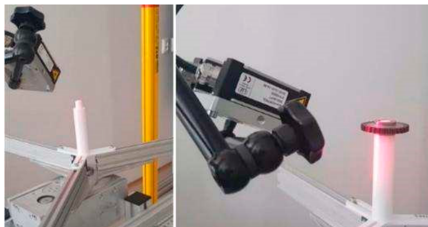
Figure 2. The experimental inspection laboratory stand; first step (left): scanning the shaft as a calibration process; second step (right): scanning the gear wheel.
