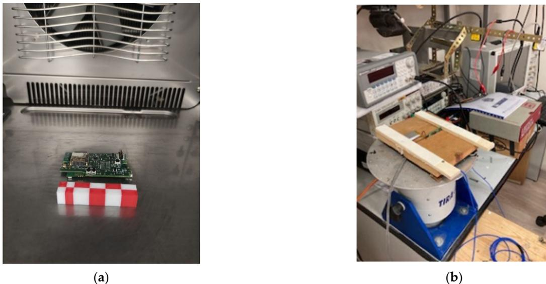
**Figure 5.** Experimental setup used in laboratory to characterize the IoT-based measurement system: (a) sensor inside climate chamber for relative humidity and temperature, (b) sensor on copy structure on the shaker.
