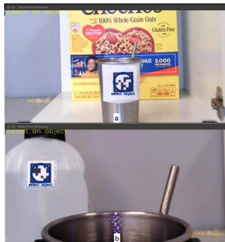
**Figure 3.** The touchscreen displays an object selection GUI overlaid on the gripper’s camera view. (a) shows tag detection with a blue selection circle highlighted to initiate a cup grasp, and (b) shows a selectable blue circle that initiates automatically moving the ARM to a jug fill position.
