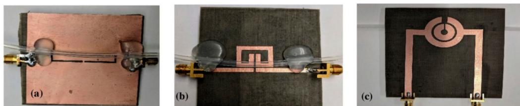
**Figure 10.** The geometries of the proposed three sensors, based on the complementary split ring resonator (CSRR) (a), extended gap SRR (EX-SRR) (b), and circular SRR (c) [98]. Reprinted from Sharafadinzadeh, N.; Abdolrazzagli, M.; Daneshmand, M. Investigation on planar microwave sensors with enhanced sensitivity from microfluidic integration. *Sensors Actuators, A Phys.* **2020**, *301*, 111752, doi:10.1016/j.sna.2019.111752 with permission from Elsevier.
